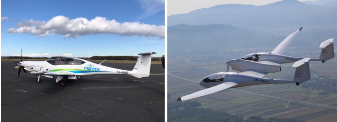
Fig. 1: the Hybrid Electric Pipistrel Panthera (left) and the Fuel Cell Hybrid Pipistrel HY4 (right)
