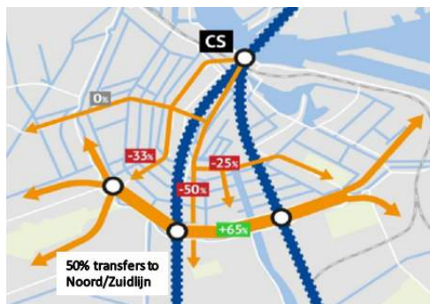
Figure 3.8: Proposed change in tram network in the city center. Adapted from Stadsregio Amsterdam (2014). Orange = tram, blue = metro.
