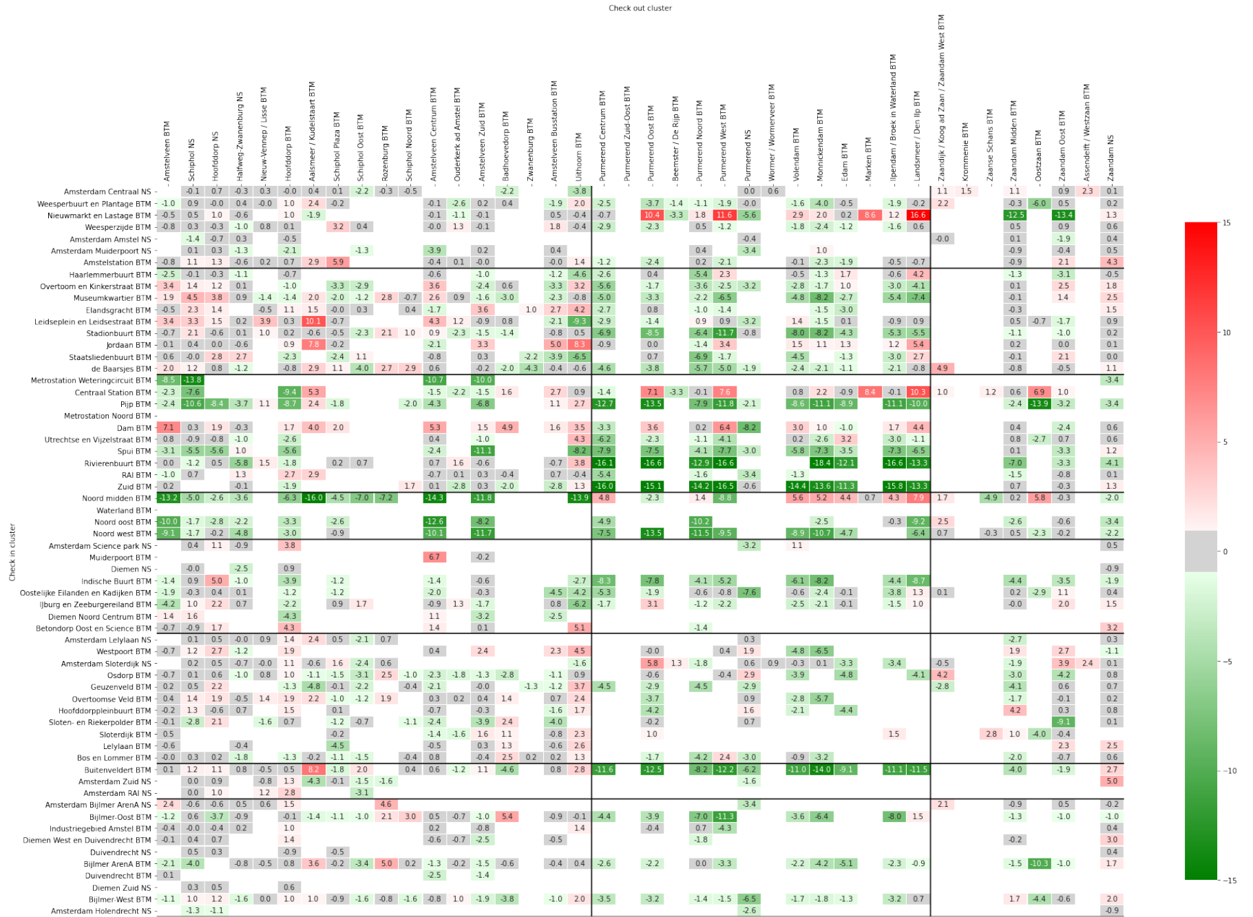
Figure V4: The absolute change in travel time for OD-relations from Amsterdam to the region over the whole day. The representativeness criterion is 51.
