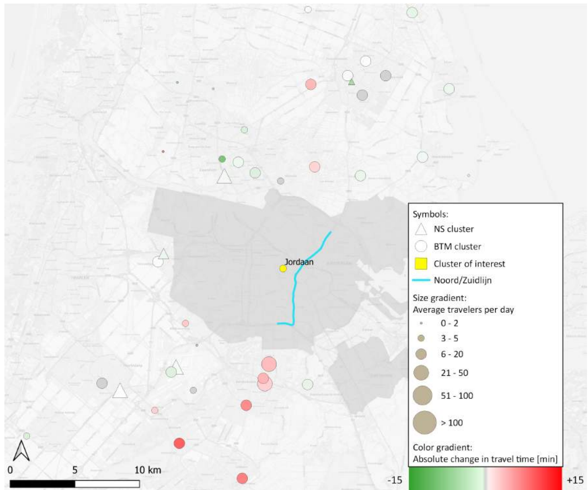
Figure 5.10: The absolute change in travel time from the regional stop clusters to Jordaan
