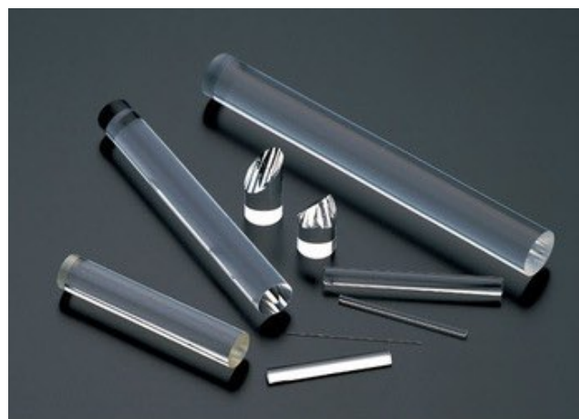
Figure 3.4: Rod lenses of different sizes, including two broken pieces.
