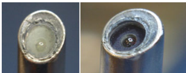
Figure 3.2: Damaged and dirty distal windows
