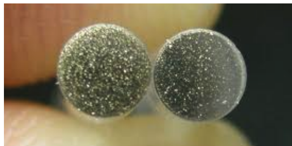
Figure 2.4: Brass flakes on rod lenses
