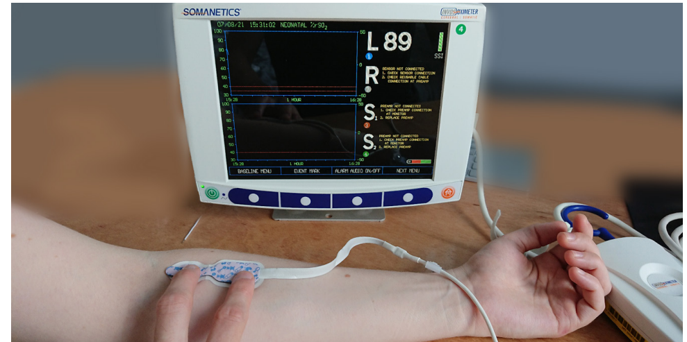
Figure 24. Invos tissue oximeter, showing 89% oxygen saturation in the anterior region of the forearm.
