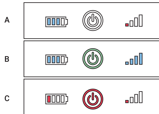
Figure 40. The user interface will light up the battery indicator and signal strength indicator when turned on (A). When the signal strength is high and the battery level is high enough, the device will start measurements and the on button will turn green (B). In case of an error or low battery, the on button will turn red (C).
