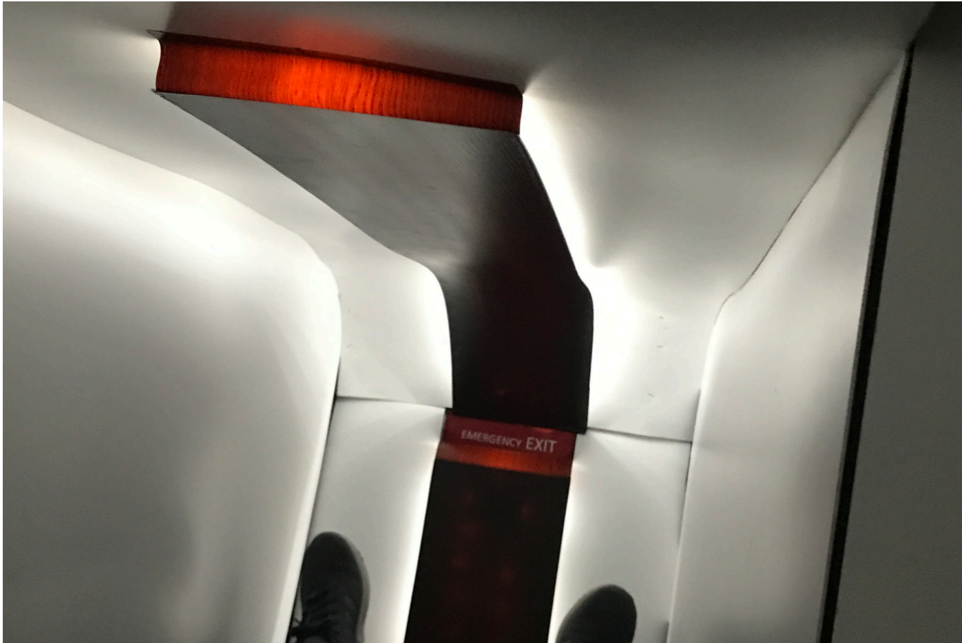
As can be seen, the wooden foil is transparent to some extent. This has been solved for the final user test with the aid of dark tape that has been stuck on the other side. The result was that the wood appeared more like wood instead of foil.
