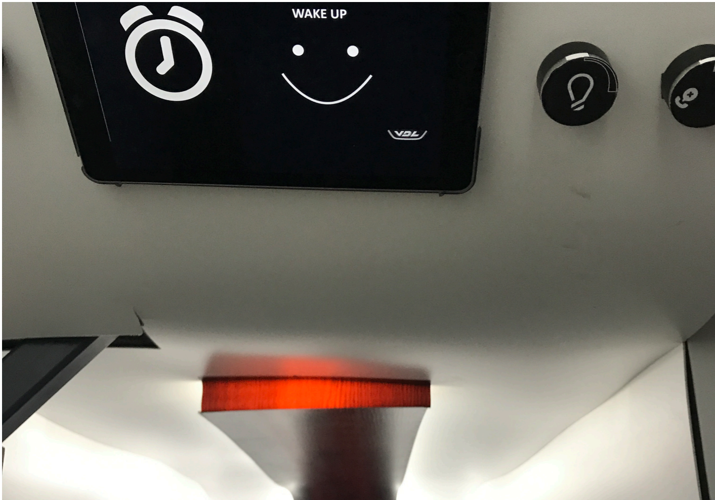
As can be seen, the wooden foil is transparent to some extent. This has been solved for the final user test with the aid of dark tape that has been stuck on the other side. The result was that the wood appeared more like wood instead of foil.
