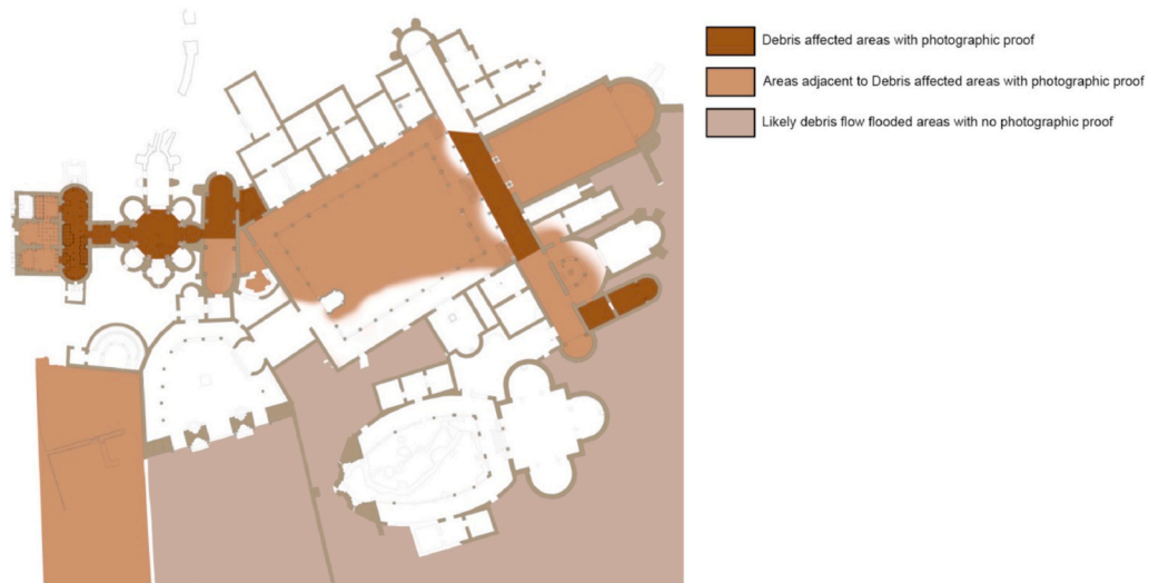
Fig. 7. Map of areas flooded in 1991. In dark brown areas with debris on the mosaics recorded through photos; in mid brown adjacent areas, which very likely have been invaded by debris, even if there are no photographs; in light brown areas likely invaded by debris, because of their geomorphological features.
