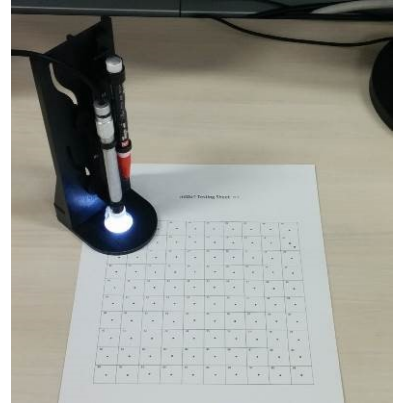
Fig. 6. Experimental setup to test accuracy of dot tagging and identification.
