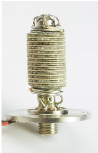
Figure 3.4: Joule-Thomson cryocooler by LeTehnica, 2023
