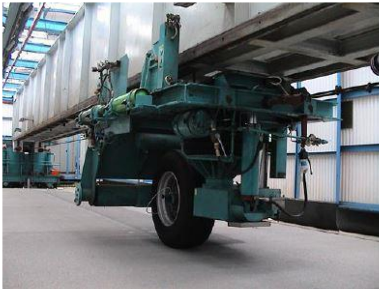
Figure C1. LINTRACK device with wide base tire.
