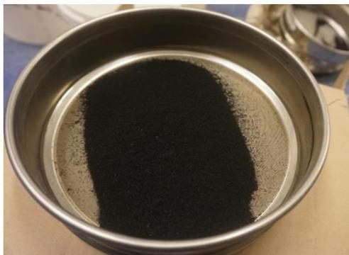
**Figure 5.1** Appearance of crumb rubber with particle sizes ranging from 0~0.71 mm.
