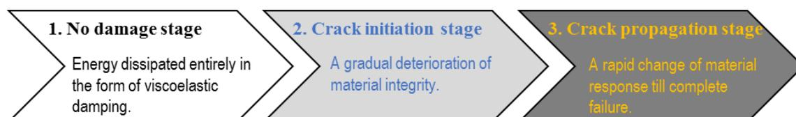
**Figure 6.7** Fatigue damage evolution of binders.
