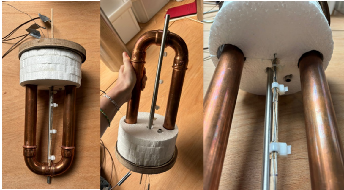
Four thermocouples are attached with tie wraps and glue to the placeholder stick in the buffer reservoir (1L, 2L, 4L & 6L depth in the reservoir).
