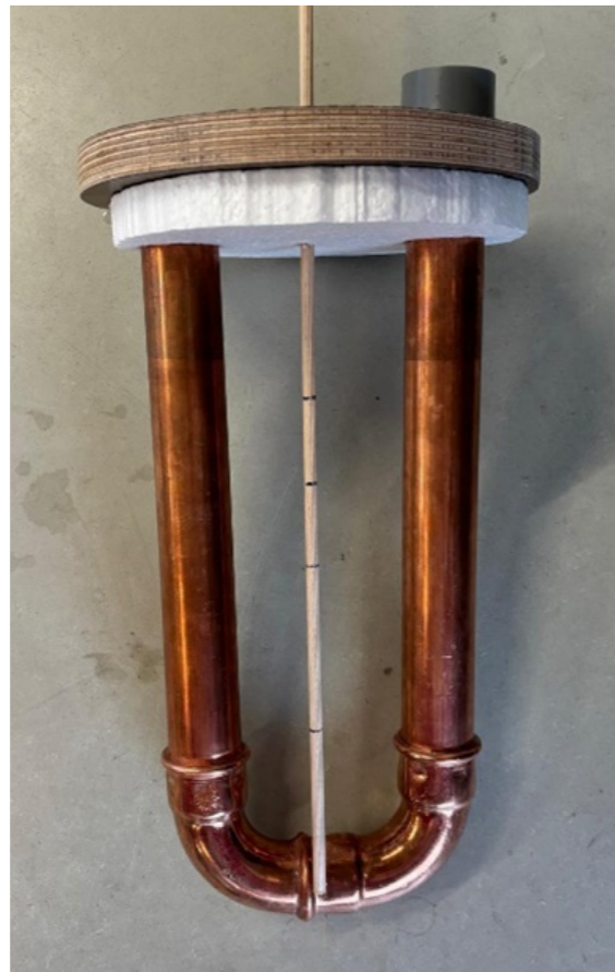
(Figure 42: U-shaped prototype with placeholder stick)
