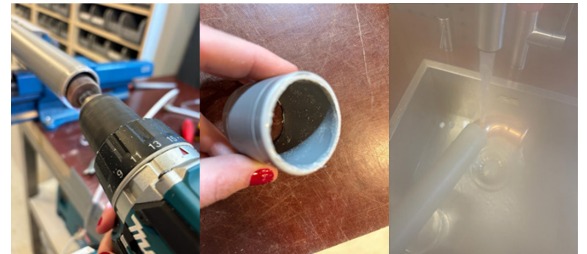
Shaping & thermoforming PVC tube (diameter 40 mm) around copper tube (diameter 35 mm)
