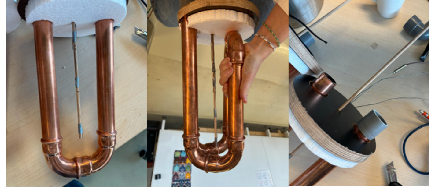
Placing thermocouples in the prototype on 1, 2,4 & 6 L depth:
