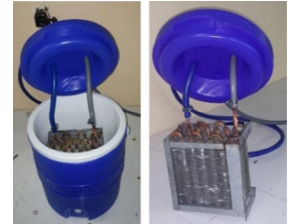
(Figure 27: Fin and tube heat exchanger in heat exchange tank (Selimli et al., 2019).)
