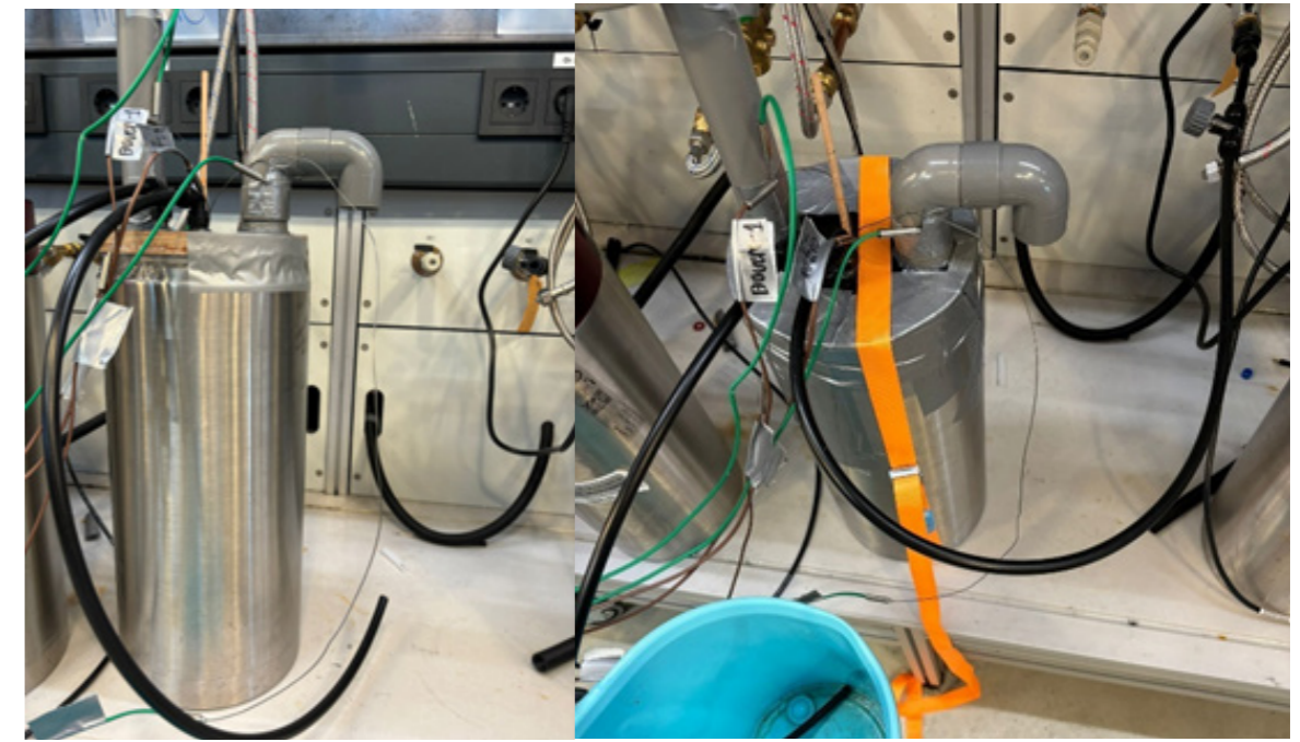
An additional layer of duct tape and a strap was added around the lid of the prototype to limit the chance of water leakage during the final test. The inlet tube was attached to a needle valve and attached to the cold water net through a screw-in coupling.
