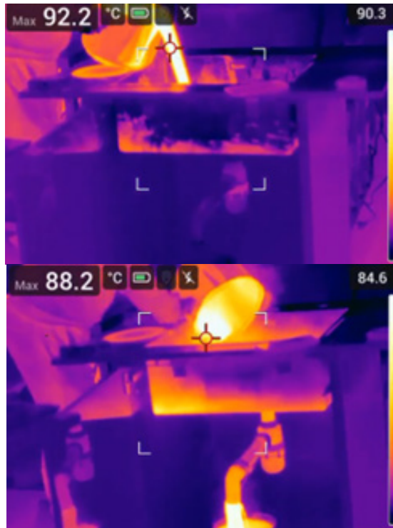
(Figure 19: explorative temperature test of draining 5 L of boiling water)
