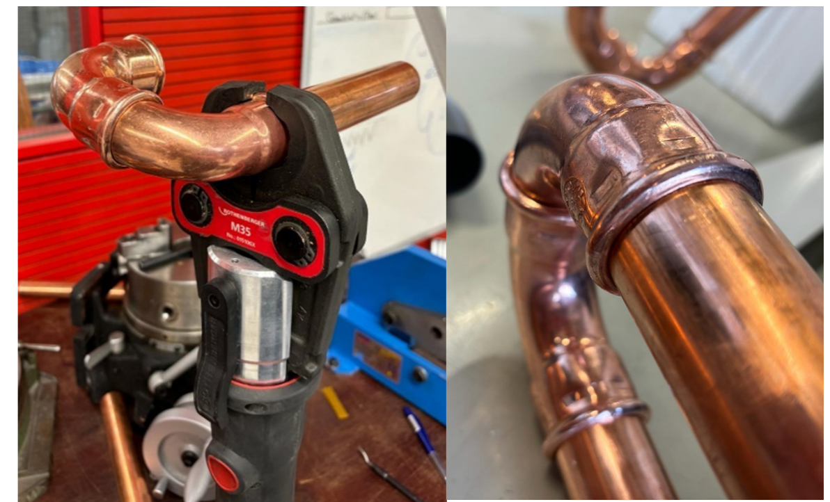
(Figure 40: attaching the parts by a press jaw)
