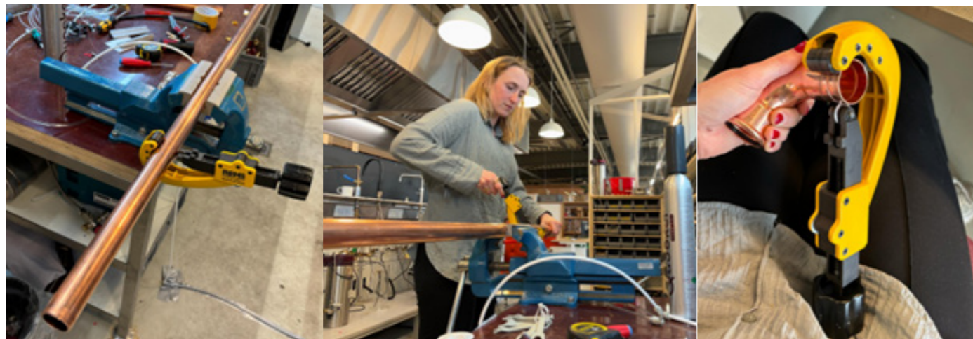
Cutting the tube and bends into desired dimensions
