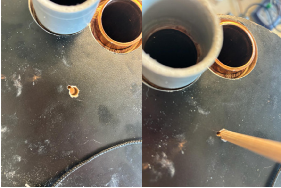
Wooden placeholder attached in the lid with HEX system:
