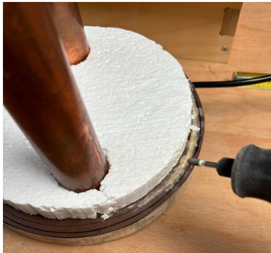
Making a rough surface on the lid so that the glue will better adhere to the surface.
