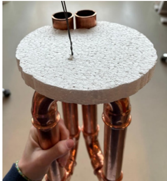
(Figure 41: W-shaped prototype with PS insulation & wire to carry the weight of the tube)
