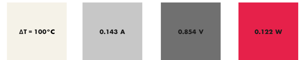
(Figure 21: Outcomes Seebeck effect of connecting boiling water and ice cold water to a Peltier element based on an experiment of RimstarOrg (2013))the CUBE)
