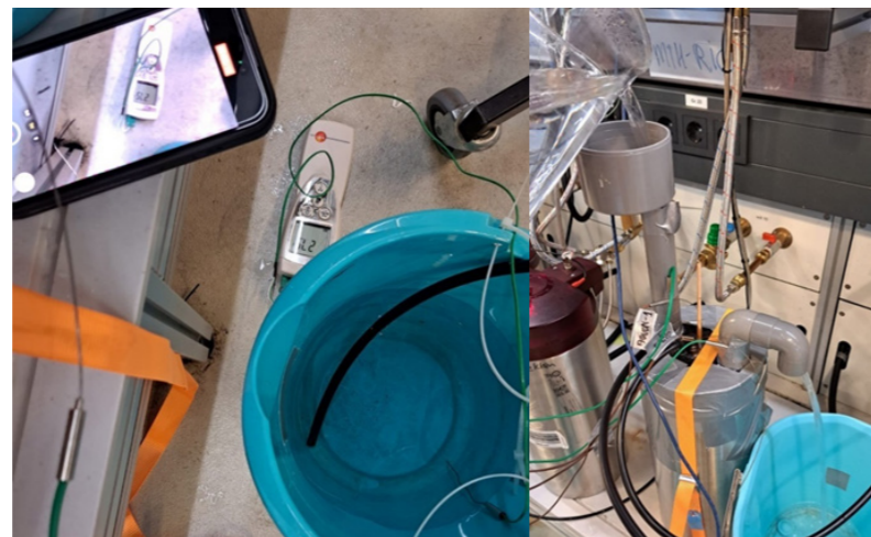
(Figure 55: test set-up & measuring water from outlet buffer reservoir)
