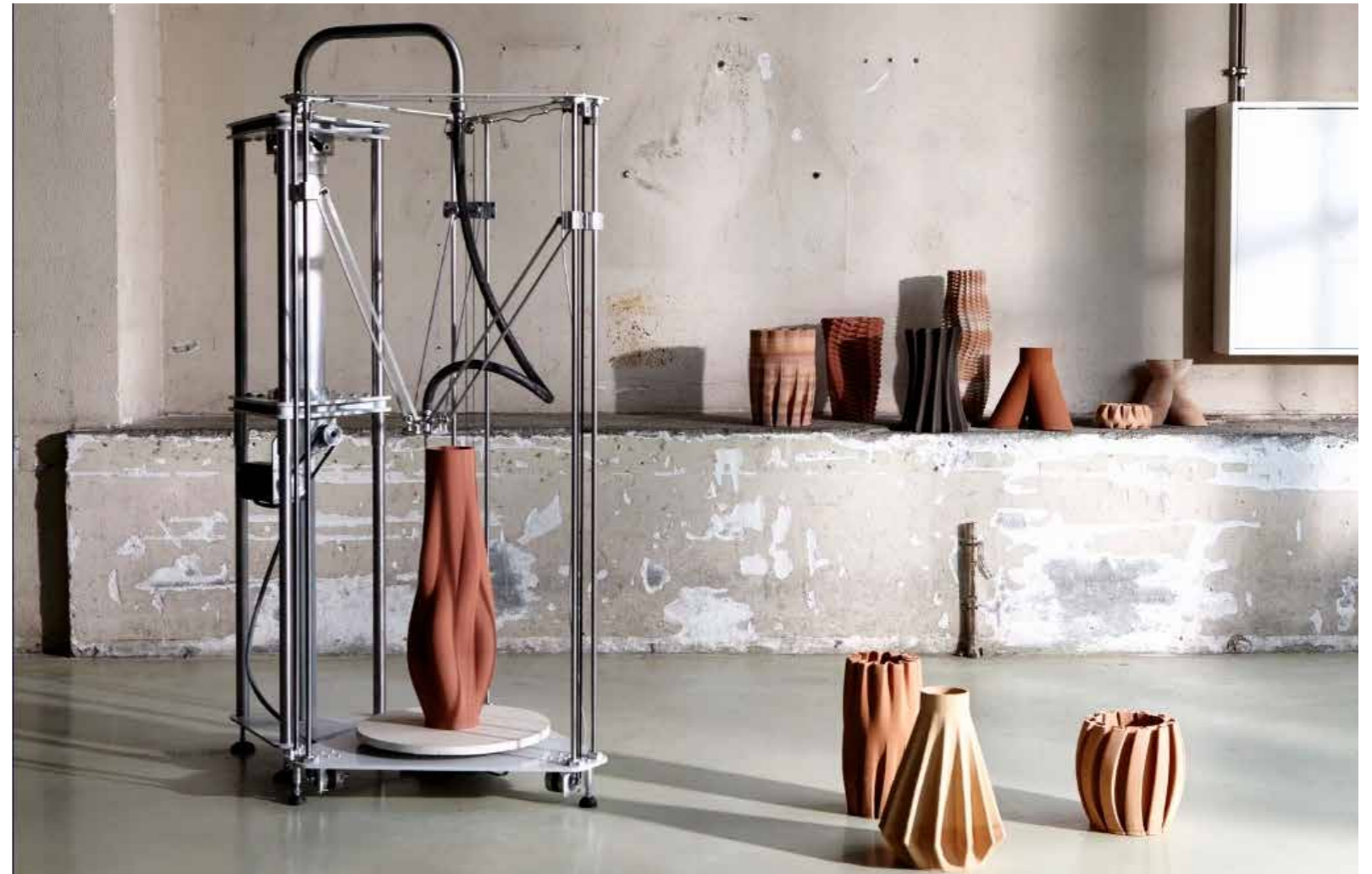
Ceramic-porcelain-3d-printer by Olivier van Herpt Logo https://oliviervanherpt.com/blue-and-white-porcelain/
