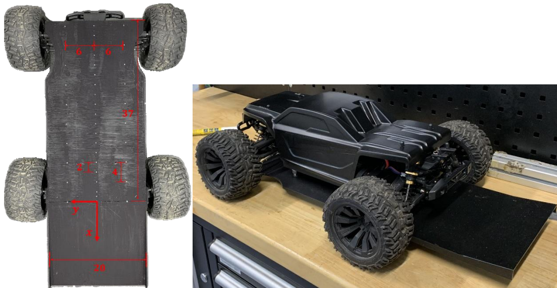
Figure 2. Pictures of the RC car. Left: underbody with markers and annotated dimensions in cm. Right: RC car with 5° diffuser.
