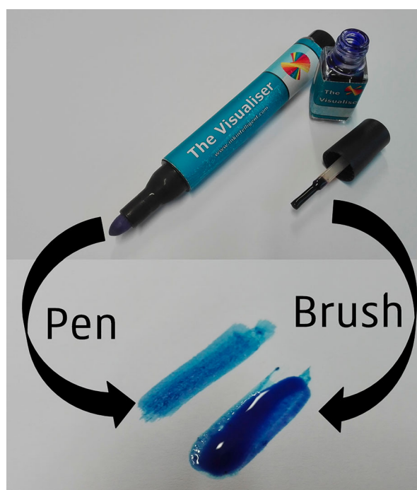
Figure 1. Photograph of the visualizer pen and brush (top) and their application on paper (bottom). The pen was chosen in this study for its dry and therefore more reproducible application.
