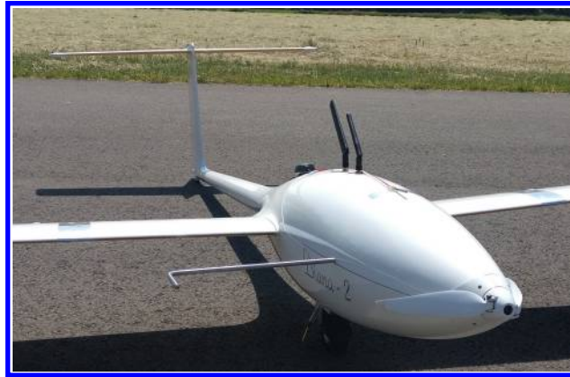
Fig. 22 Aeroprobe installation location.
