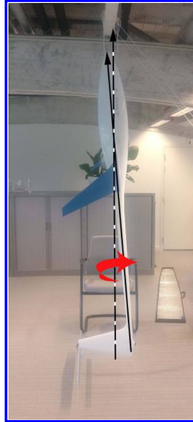
Fig. 5 Roll moment of inertia setup.
