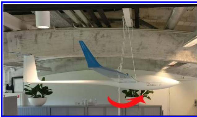
Fig. 2 Pitch moment of inertia setup.
