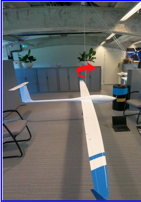
Fig. 4 Yaw moment of inertia setup.
