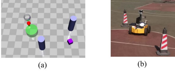
Fig. 2. (a) Simulation scenario in Safety Gym: The objective is to move the vehicle (red) to the green region while avoiding two static obstacles (grey), the moving soft object (purple) is not considered in the controller design. (b) Experimental platform of the differential-drive vehicle and testing scenario.
