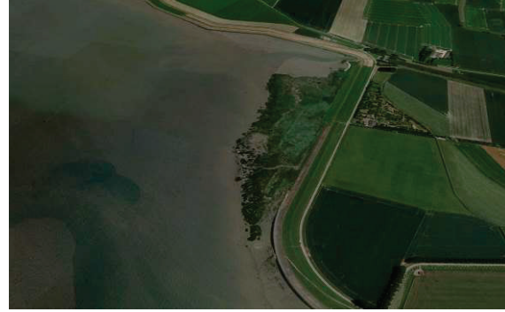
Hellegat, salt marsh, Western Scheldt Marsh elevation 3.0 m+NAP, width 200 m, slope 1:40 Dike height 9.5 m+NAP, slope 1:4 Design conditions: h = 6.0 m+NAP, H_{m0} = 1.9 m, T_{m-1,0} = 5 s
