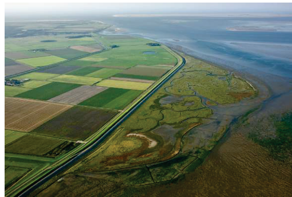
Texel, salt marsh Schorren, Wadden Sea Marsh elevation 1.8 m+NAP, width 400 m, slope 1:250 Dike height 6.9 m+NAP, slope 1:3 Design conditions: h = 4.4 m+NAP, H_{m0} = 1.4 m, T_{m-1,0} = 5 s
