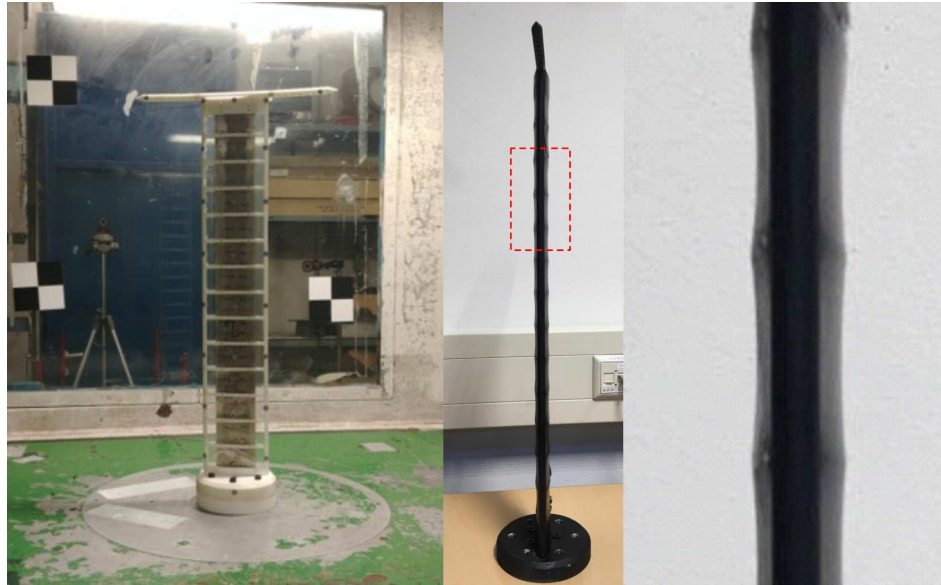
Fig. 1 Pazy Wing in wind tunnel at Technion (left) [1]. Outer surface of the Pazy Wing from TU Delft in undeflected jig-shape with close up highlighting the sagging skin (foil cover) between the ribs.
