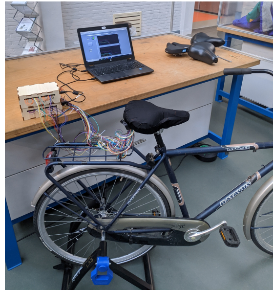
Fig. 9. Test setup used during the saddle test.
