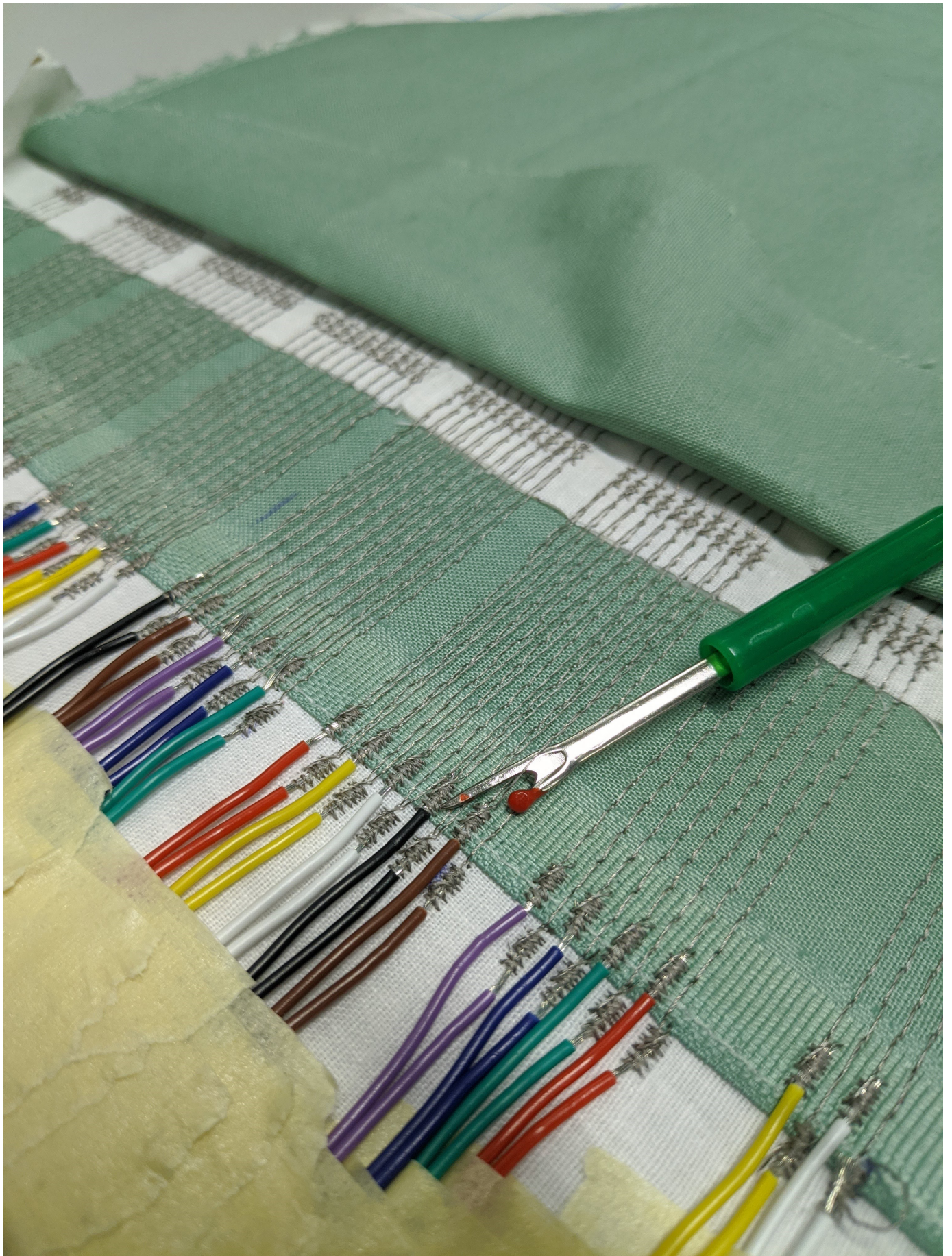
Fig. 5. Transition from conductive threads to usual electrical cables
