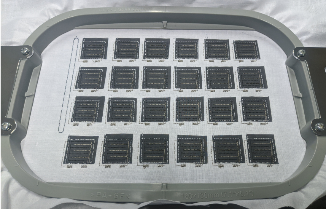
Fig. 1. A batch of 24 sensors right after the embroidery process.
