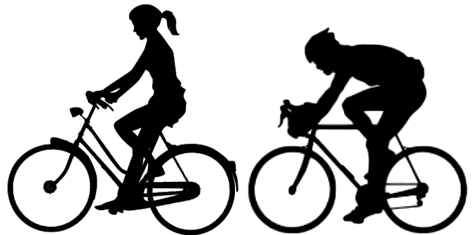
Fig. 1. Postures adopted while using a city bike [11] (left) and a road bike [12] (right).
