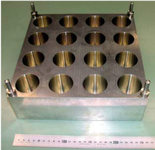
Figure 3.19: Mould for small size electrodes, bottom part.
