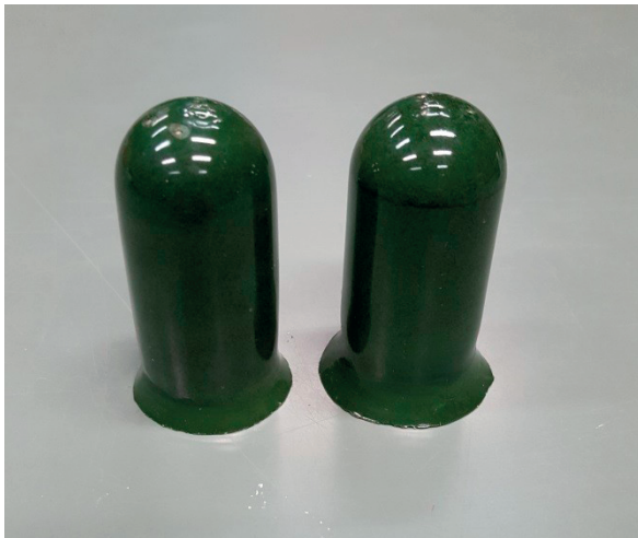
Figure 3.13: Semiconductor A coated small size electrodes.
