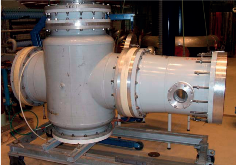
Figure 3.1: Picture of test setup GIS enclosure
