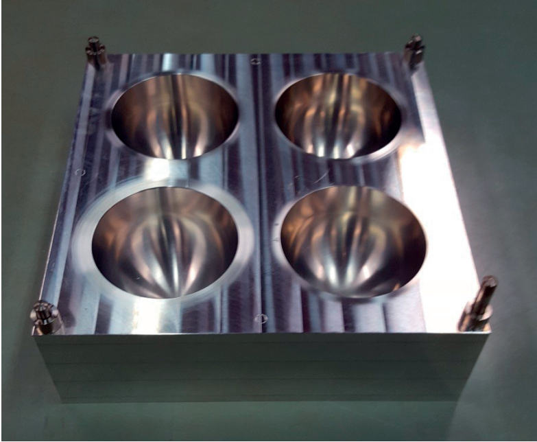
Figure 3.21: Mould for large size electrodes, bottom part.
