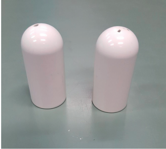
Figure 3.12: PA11 coated small size electrodes.
