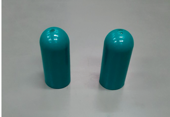
Figure 3.7: EP-I coated small size electrodes.
