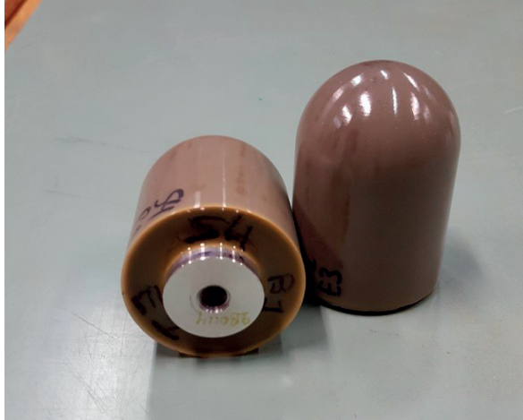
Figure 3.17: Nanocomposite B coated small size electrodes.
