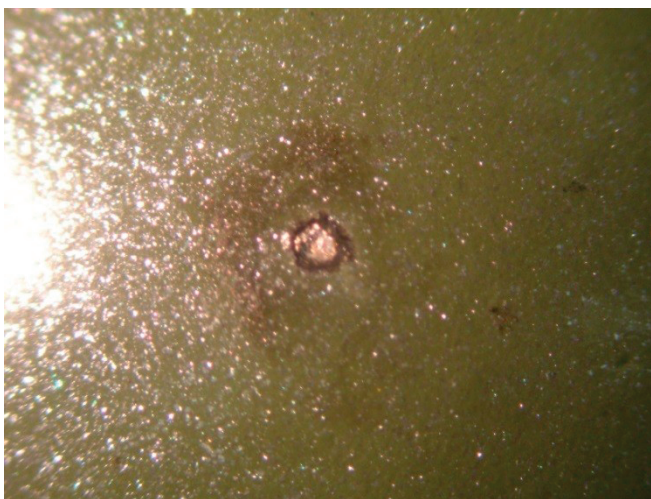
Figure 5.40: Microscopic view of the surface of a FP-IV coated electrode after a breakdown test.
