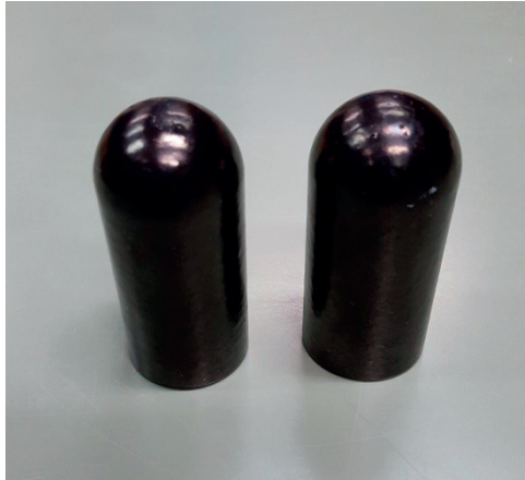
Figure 3.9: FP-II coated small size electrodes.
