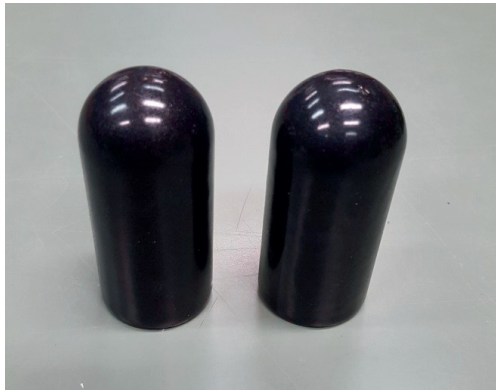
Figure 3.14: FP-II + FP-I coated small size electrodes.
