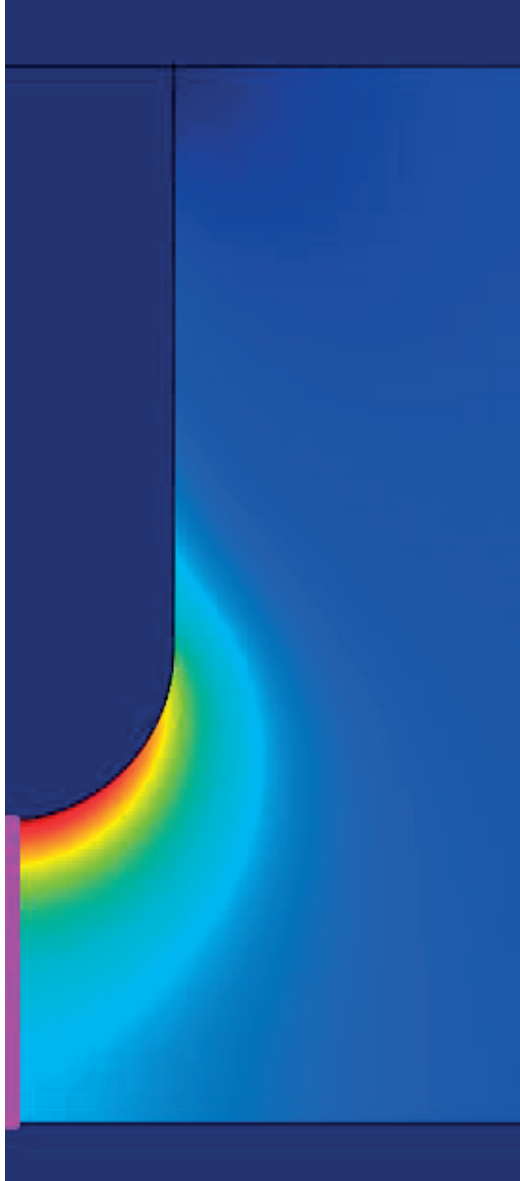
Figure 6.2: 2D rotational symmetric electric field calculation in rod-plane gap. The purple line represents the evaluation line.
