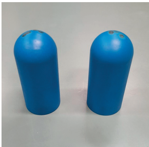
Figure 3.10: FP-III coated small size electrodes.
