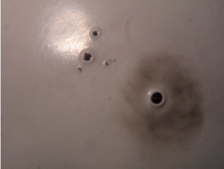
Figure 5.38: Microscopic view of the surface of a PA11 coated electrode after a breakdown test.
