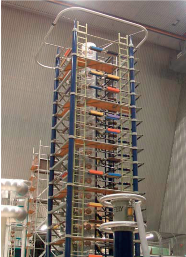
Figure 3.29: 20-stage Haefely impulse voltage generator.
