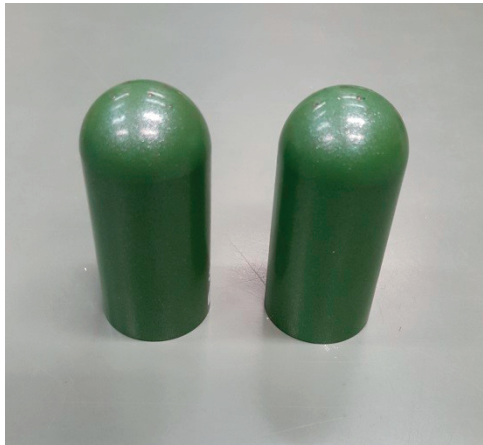
Figure 3.11: FP-IV coated small size electrodes.
