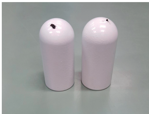
Figure 3.15: FP-II + PA11 coated small size electrodes.
