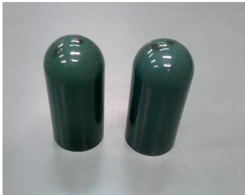
Figure 3.8: FP-I coated small size electrodes
