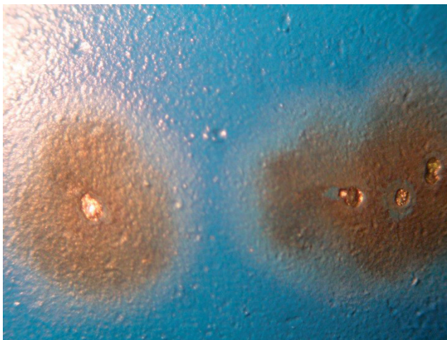
Figure 5.41: Microscopic view of the surface of a FP-III coated electrode after a breakdown test.
