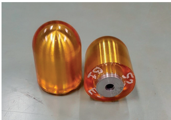
Figure 3.16: Neat epoxy coated small size electrodes.
