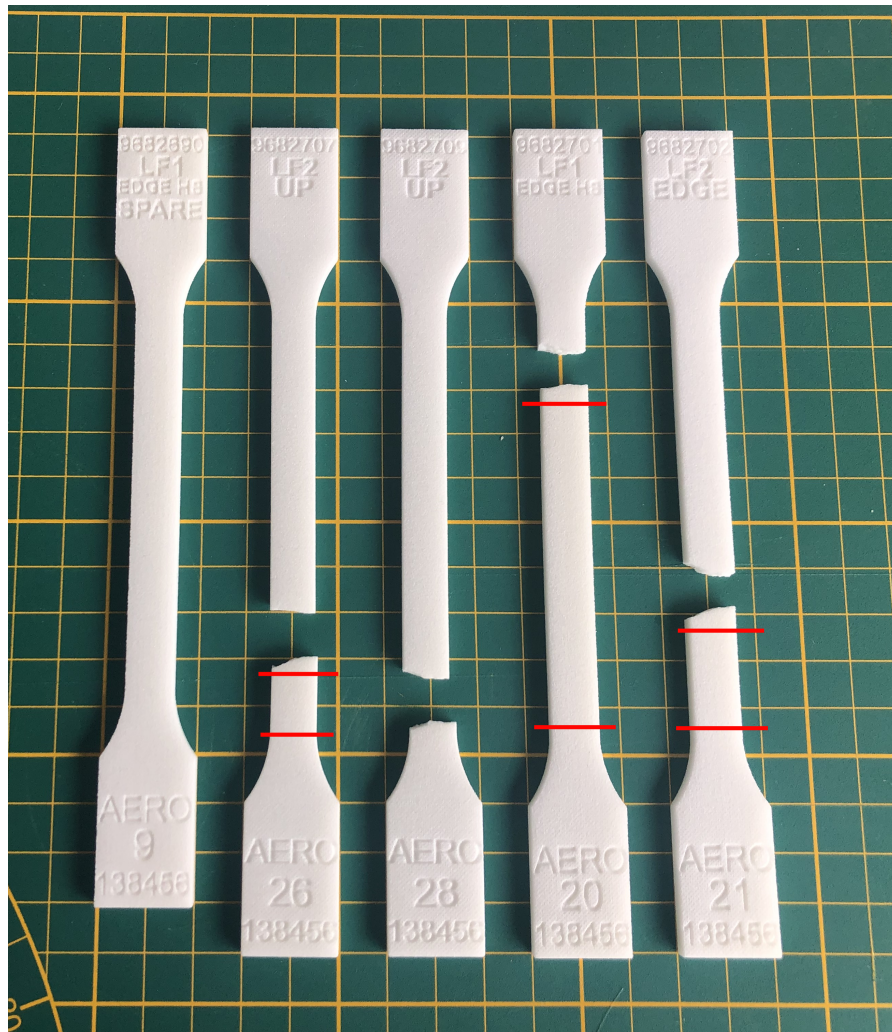
Figure 5.2: Example of tensile specimens cut for the use as an estimation of the porosity
