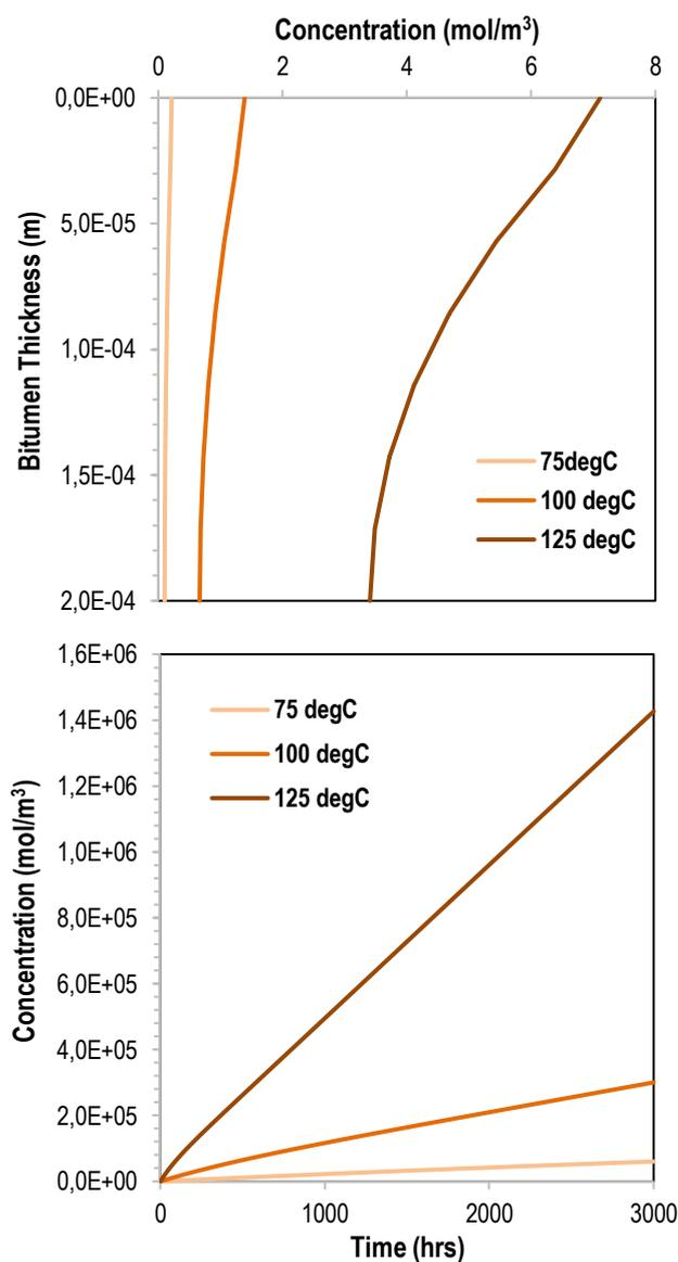
Figure 3. Predicted concentration of oxidized species along the thickness after 3000 hrs (top) and in bitumen (bottom).
