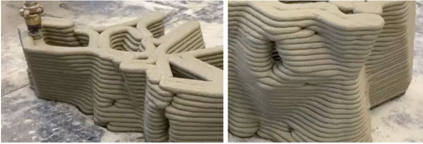
Fig. 3.1 Rhizome 1.0 prototypes using Vertico's cement-based concrete and robotic system
