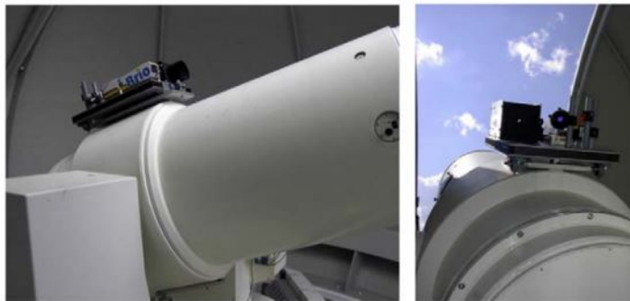
Figure 9.1: BELA mounted on the telescope at the Wettzell ground station in south Germany (Schreiber et al., 2009)
