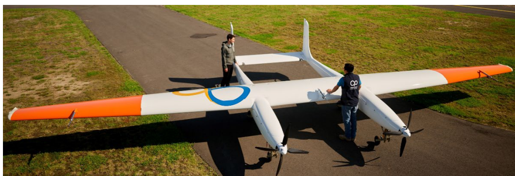
Figure 3. Ampyx Power's AP3 during flight testing on Breda International Airport in May 2021 (photo courtesy of Ampyx Power B.V.).
