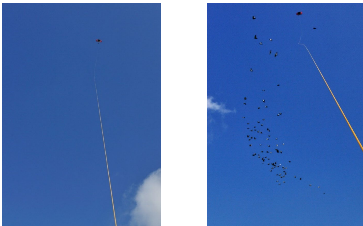
Figure 5. Pilot operation of the 20 kW kite power system of TU Delft [88] before (left) and after a bird collided with the tether (right). The bird continued the flight seemingly unaffected, which suggests that bird collisions with a tether are possible but do not necessarily have to be fatal. Max Dereta took the photos on 28 June 2011 at Valkenburg airfield, The Netherlands.
