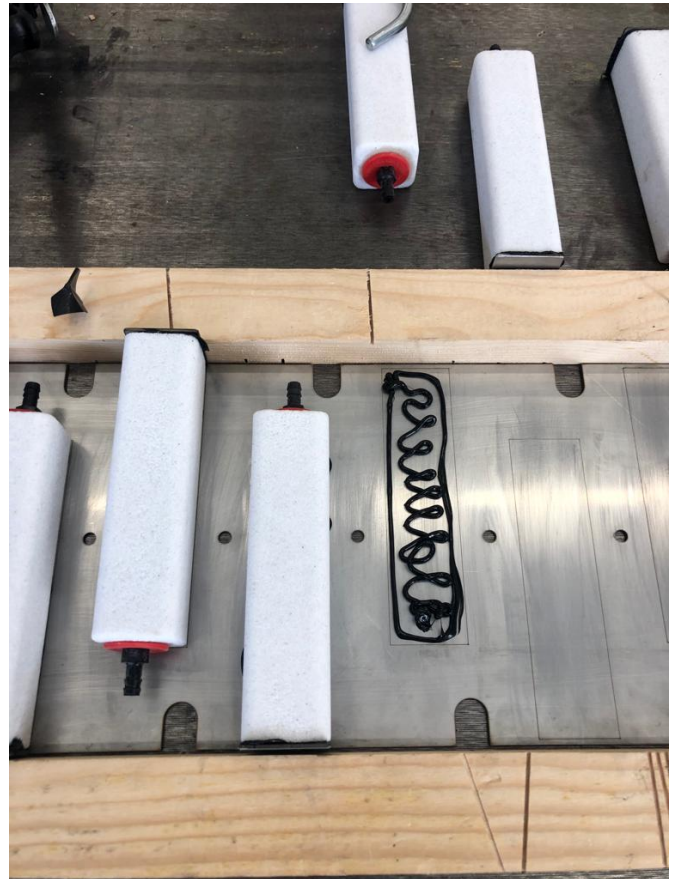
(b) On both sides of the bottom placed a wooden support is places so the aeration stones wouldn't accidentally move during the glue process. When the stone would move and will be sticking out at the outside border, the bottom plate will not fit in the tank any more
