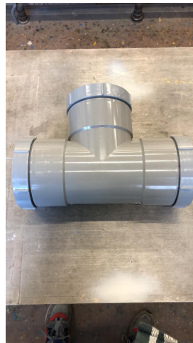
Figure 15: A 3.2[mm] thick rainpipe with a diameter of 125[mm] is used as a air manifold. The main reason for the manifold is to distribute the air as evenly as possible over the 10 different air hoses.
