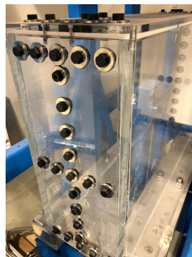
Figure 8: In this figure, the cable entries are visible. These old cable entries are on both sides of the tank. For this new tank design, the cable entries will be used for supporting purposes only
