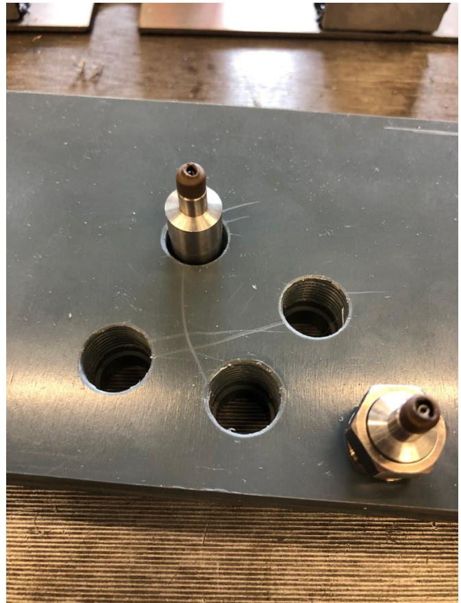
(b) The top plate has a m14 fine tread in the material so the sensor can be screwed in to place. This special hollow bolt, is designed for the sensor and prevent the sensor from moving upwards when a wave hits the overhang and the sensor.
