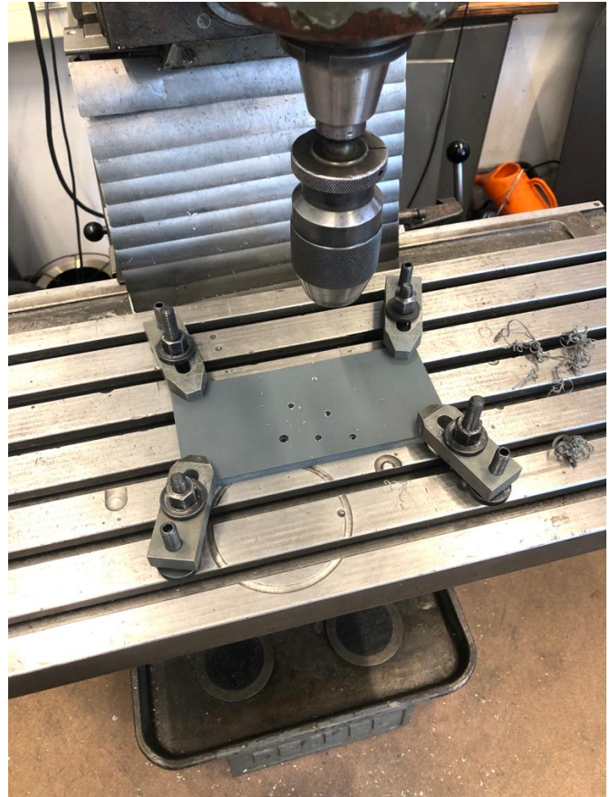
(b) Because the second plate needs a m14 fine thread, the plates could not be glued first and drilled after. This is the reason that it is done at a milling machine with a digital measuring system with an accuracy of 1/1000 mm
