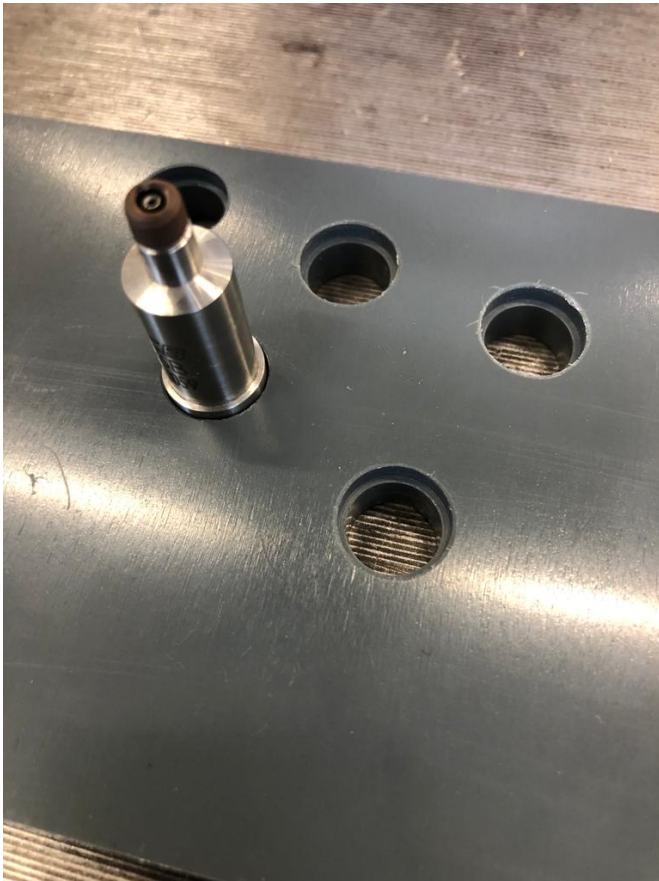
(a) The bottom part of the sensor plate is a plate with a precise fit for the bottom part of the sensor. This has extra edge cut out of the material so the sensor will fit in perfectly. This extra edge is designed so the sensor can not fall trough the object.
