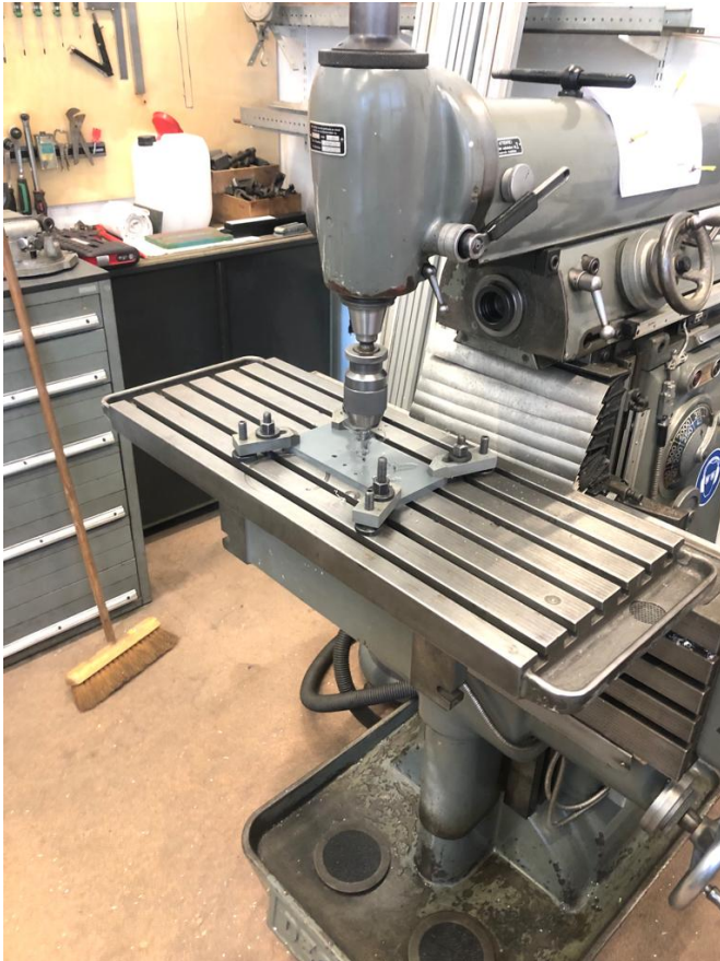
(a) The drilling of the holes of the sensor is done at the milling machine. This is done because the 2 plates need the center of the sensor holes exactly on the same location.
