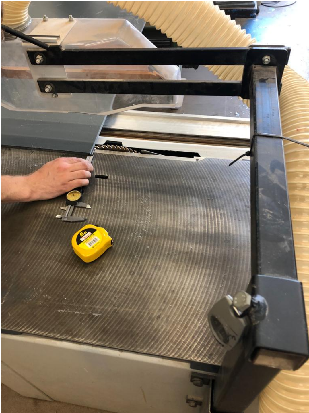
Figure 42: With no accurate measuring system of the saw it self, all the measuring must be double checked by hand.
