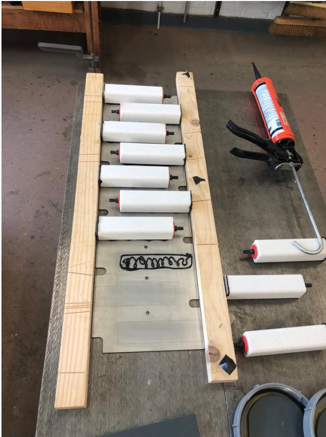
(a) The glue is evenly distributed at the plate and at the stone, at all times there is one line of glue at the outside border of where the stone will be, this so any air leak will be sealed off.
