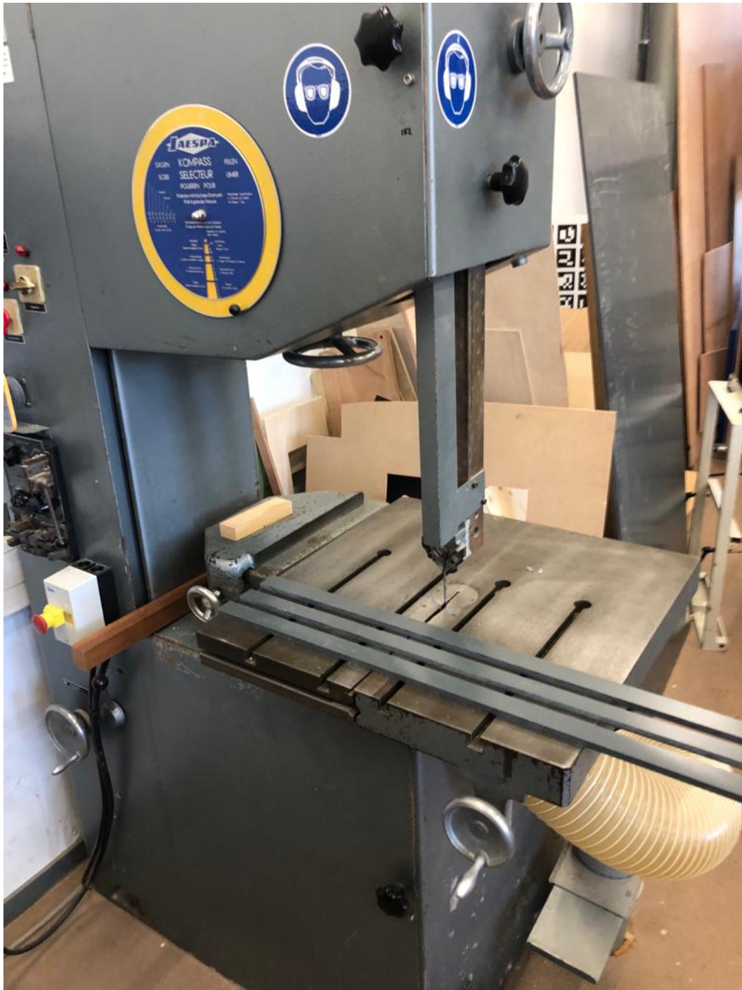
Figure 43: For smaller saw cuts, the bandsaw was used. Cutting in a straight line is more difficult, so only the small cuts were done here
