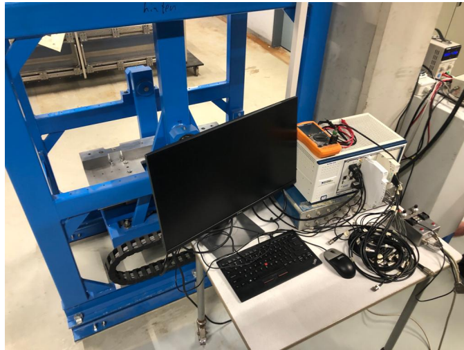
Figure 17: The computer that is coupled to the experimental setup performs two functions. The first function is to send a control signal with the desired frequency to the drive motor of the tank. The second function is to receive all the data of the different sensors.
