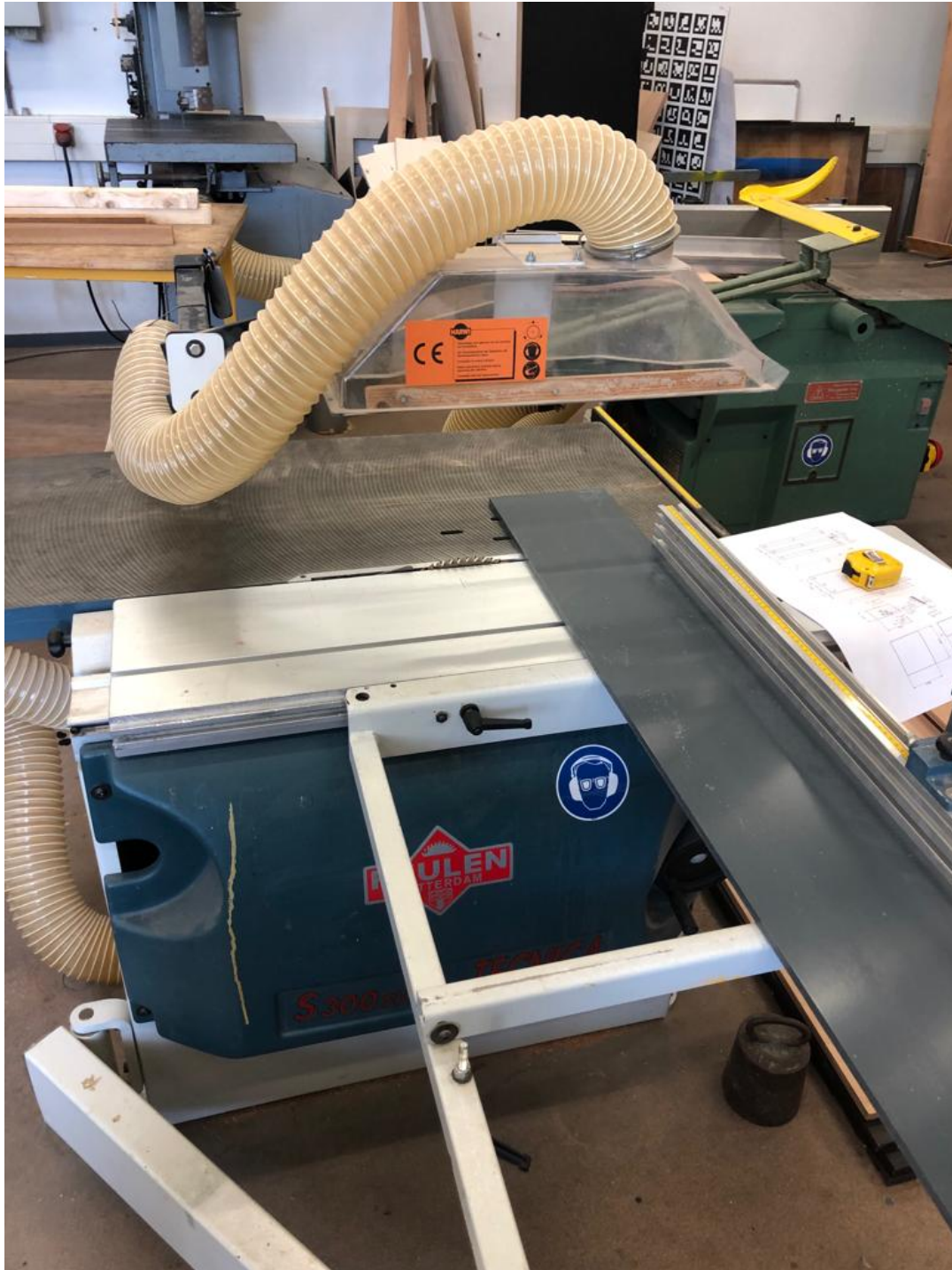
Figure 41: The overhang construction is made from Polyvinyl chloride. This was ordered as a 1[m]x2[m] plate with a thickness of 10[mm]. The first plan was to laser cut this plate as well. This would be very accurate and time efficient. But due to unforeseen limitations of the laser cutter, the construction must be saw by hand with the table saw.
