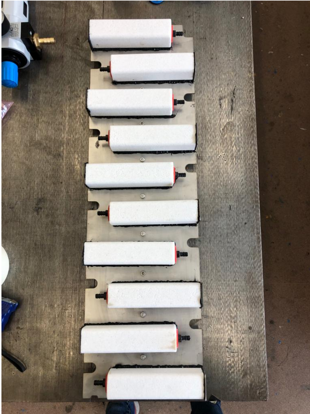
Figure 48: The end result of all aeration stones glued to the bottom plate. The advice of the glue manufacture was followed, and the stones were not loaded with any force for 48 hours
