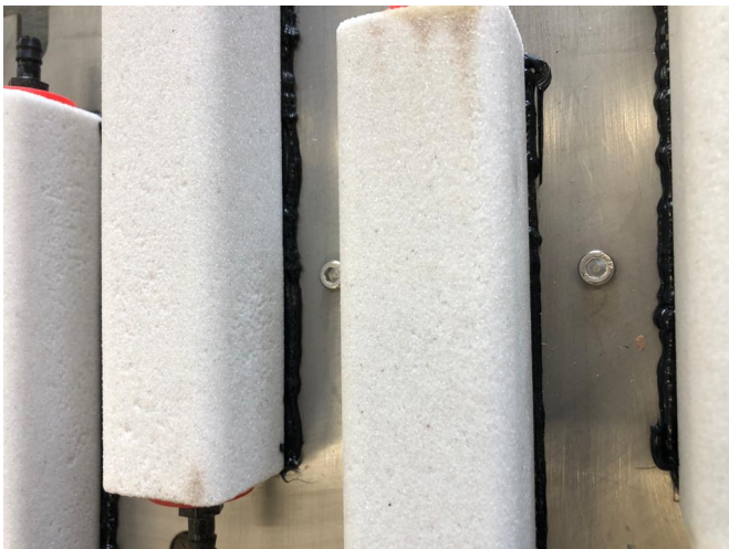
(a) The bottom part of the aeration stone is sealed with a extra fillet of glue. This to prevent air escaping from the bottom side of the stone
