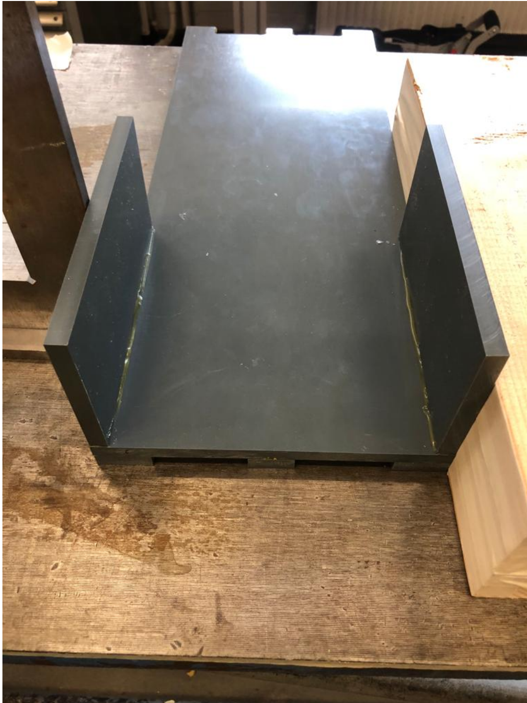
Figure 51: The gluing process started with the back plate and the 2 side walls, these were supported by 2 exactly 90 degrees objects so the construction did not become wider than the tank.
