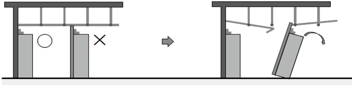
Figure 39: Heavy furniture fixed to a partition wall which was installed after the ceiling work may damage the wall and the ceiling and overturn during an earthquake.
