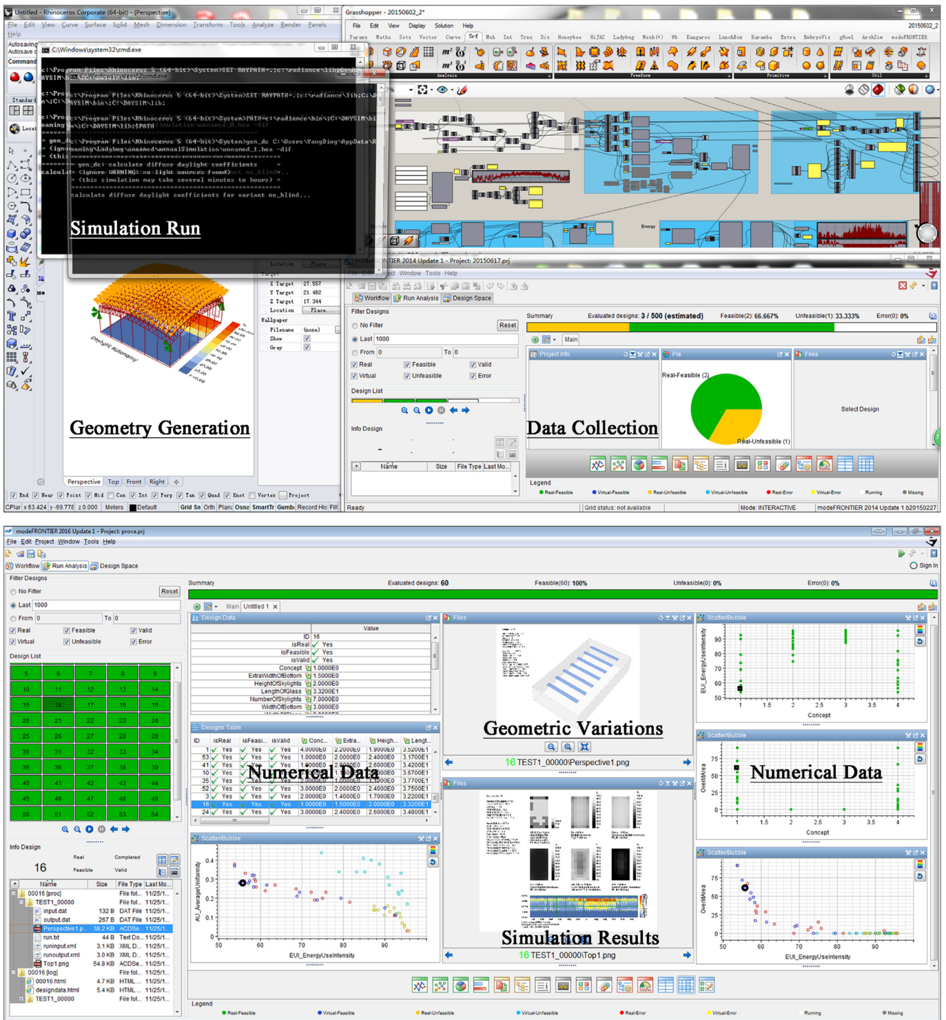
Fig. 5. Interface for process automation, i.e. automating the iterative processes of geometry generation, simulation run and data collection (top); interface for post-processing, i.e. monitoring geometric variations while exploring numerical data and other simulation results (bottom).
