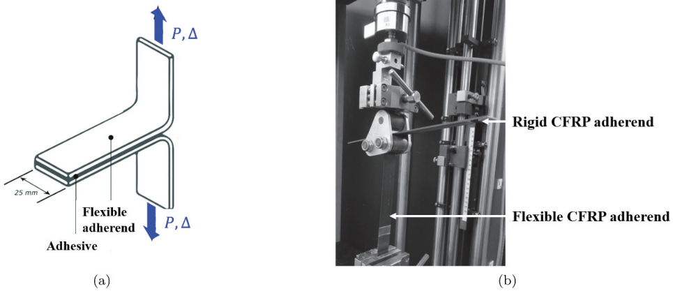
Figure 2. Schematic representation of peel testing configurations. (a) The T-peel test geometry (adopted from [25] ). (b) The Composite Peel Test (CPT) set-up (adopted from [26] ).
