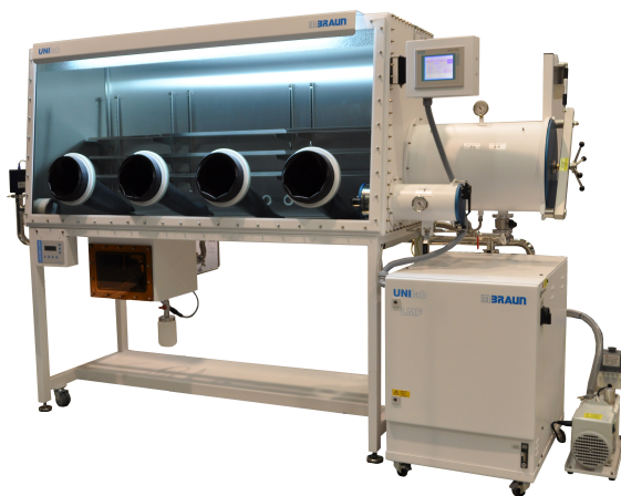
Figure 3.1: Image of the glovebox used for liquid silicon processing. Image courtesy of Salm en Kipp B.V.
