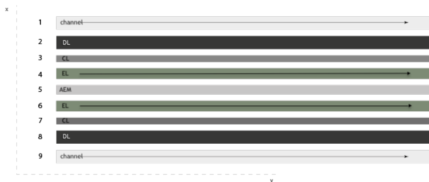
Figure 4.4: The x-y plane that is taken into account within this modeling research is demonstrated. The gas flows from left to right in the channel (1, 9), indicated with the arrow. The anode is indicated with numbers 2,3 and the cathode with numbers 7,8. The electrolyte is indicated with a green color and the numbers 4 and 6. Similar to the channel, the electrolyte flows from left to right, as demonstrated by the arrow.
