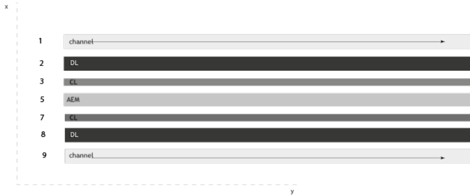
Figure 4.2: The x-y plane that is taken into account within this modeling research is demonstrated. The gas flows from left to right in the channel (1,9), indicated with the arrow. The anode is indicated with numbers 2,3 and the cathode with numbers 7,8.
