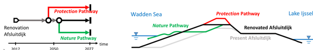
Figure 3. (Left) Adaptive pathways map for the renovated Afsluitdijk, including Protection Pathway (red), Zero Pathway (black), and Nature Pathway (green). (Right) schema of dike section showing alternative pathways.
