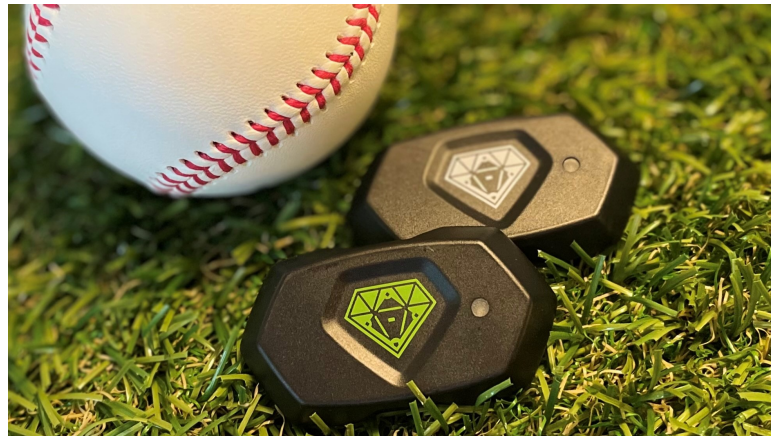
Figure 1. Pitch Perfect sensor system for measuring pelvis and trunk kinematics and separation time between them.
