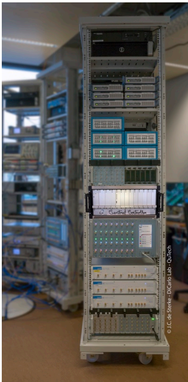
Figure 5.12: Complete quantum control system used to perform quantum computing experiments (J.C. de Sterke, QuTech, 2018)
