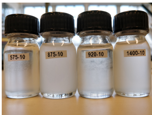
Figure 6.13: PE-b-PEG copolymers dissolved in toluene with a concentration of 10 \text{ gL}^{-1} , from left to right: B575, B875, B920, B1400.
