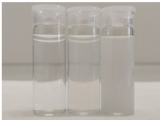
Figure 6.1: \text{H}_2\text{O}/\text{Al}_2\text{O}_3 nanodispersion diluted with ultrapure water: 100x (right), 1000x (middle) and 10,000x (left).
