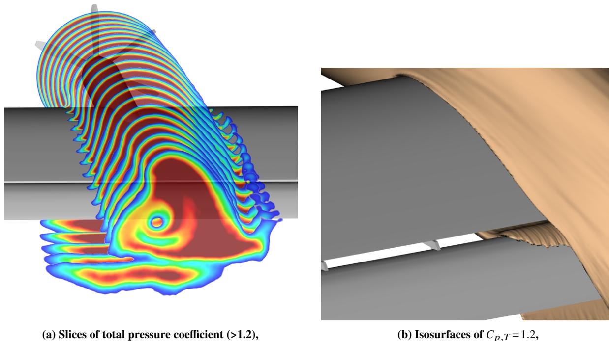
**Fig. 14** Visualisation of the slipstream deformation as it moves along the wing based on (time-averaged) total pressure coefficient  $C_{p,T}$  for the  $\delta_f = 15^\circ$ ,  $\alpha = 8^\circ$  case.
