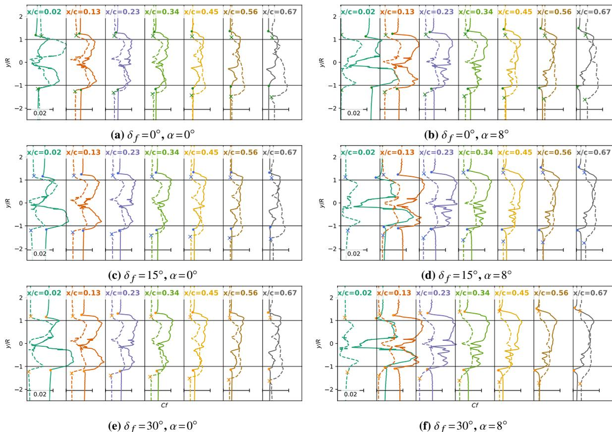
**Fig. 10** Spanwise skin friction distributions for various chordwise positions. Dashed lines are on the lower surface of the wing, solid lines are on the upper surface. Markers show the approximate edges of the slipstreams. Marker colors correspond to the lines in Fig. 11
