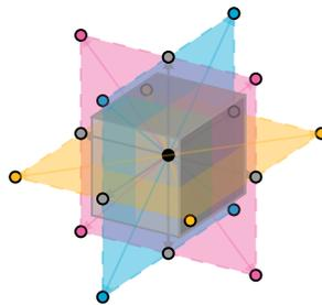
**Fig. 1 Discretization of the velocity space into 19 vectors.**
