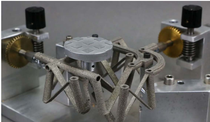
Figure 1.2: An example of a tip-tilt compliant mechanism, designed for space applications. This monolithic mechanism is made from several planar compliant modules, cross-axis flexural pivots, connected to each other with rigid elements [17].
