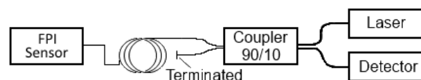
Figure 2. Schematic view of the readout system used to detect changes in the length of the elastic element in the FPI sensor. No light reflects at the terminated fiber end.
