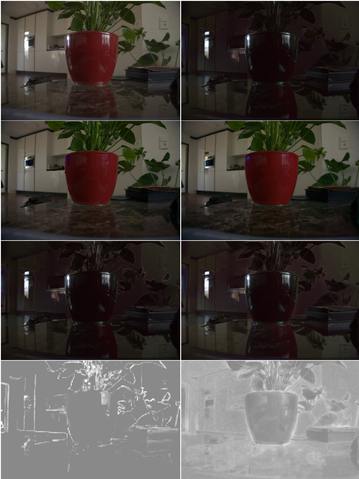
Figure 6.3: Diffuse-specular decomposition of sample set 'inside'. The top two images show I_{mean} (left) and I_{amp} (right). The next three rows have the tile-based estimate on the left, and the final decomposition on the right. Those rows show I_d , I_s and k in order from top to bottom. k is rescaled from [0, 4] into the range [0, 1] for visibility.
