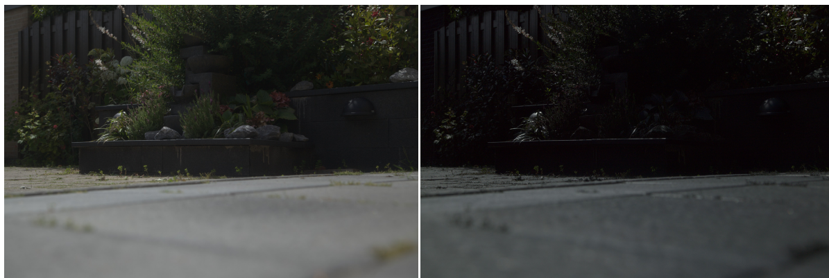
Figure 4.4: I_{mean} (left) and I_{amp} (right) for sample 'zoom'. The blue tiles on the floor are strongly polarized due to the angle of the sun, while the foliage only has polarized highlights.
