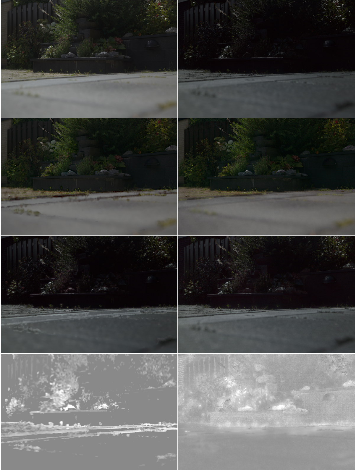
Figure 6.1: Diffuse-specular decomposition of sample set 'zoom'. The top two images show I_{mean} (left) and I_{amp} (right). The next three rows have the tile-based estimate on the left, and the final decomposition on the right. Those rows show I_d , I_s and k in order from top to bottom. k is rescaled from [0, 4] into the range [0, 1] for visibility.
