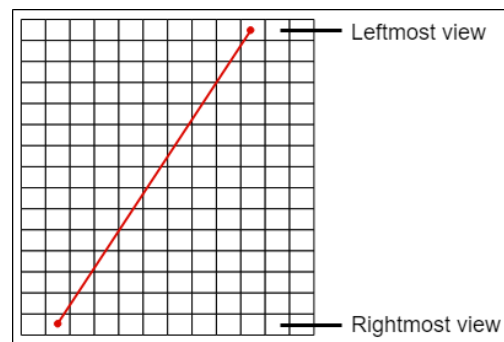
Figure 3.4. Example diagram of a single epipolar plane. Each row of pixels corresponds with a pixel row for a different view. The red line signifies one source pixel that has been transformed to its counterpart in epipolar space.
