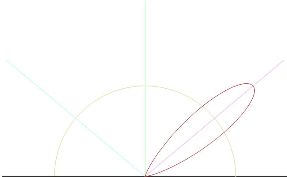
Figure 3.8. Polar plot of the reflected light distribution by the Blinn-Phong reflection model. The green line is the surface normal. The cyan line represents the incident light and is configured at 50°. The magenta line is the reflected light direction. The red lobe is the light distribution, whereby the distance from the center signifies the intensity. Source: BRDF Explorer by Disney Enterprises, Inc.
