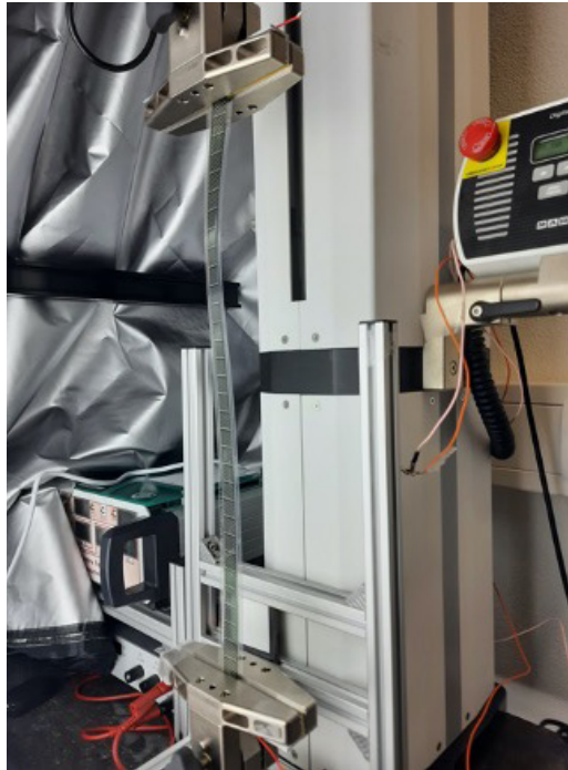
FIG. 11 OPV strip test set-up, illuminated by bright light source.
