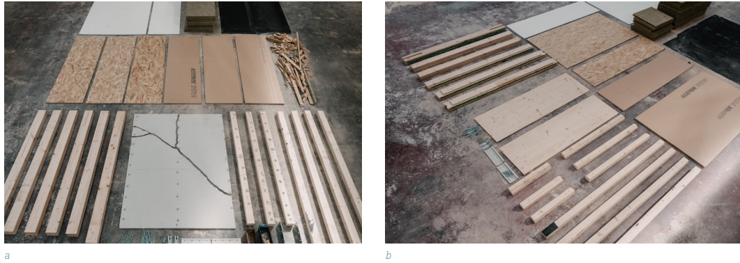
FIG. 5 Façade layers after the disassembly activity, for a prefabricated multi-layer timber-based façade joint with (a) 1_SA staples and (b) NC geometrical assembly. Images by Fiorentino.
