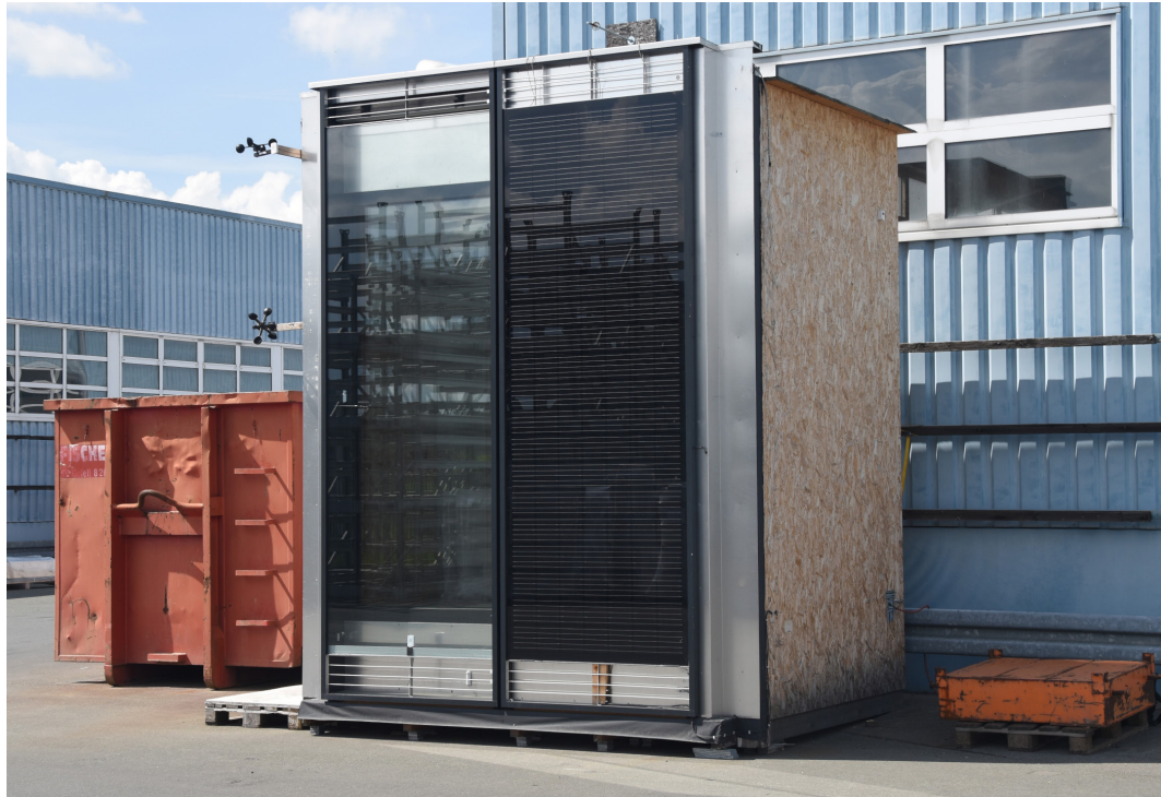
FIG. 8 PRÄKLIMA façade in front of the insulated chamber serving as a testbed for ongoing monitoring, the opaque element on the right, the transparent one left side.
