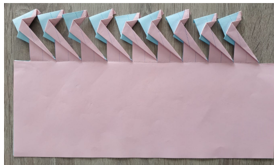
Figure K.3: Two kirigami sheets, folded into each other. The sheets are on top of each other for illustration purposes.
