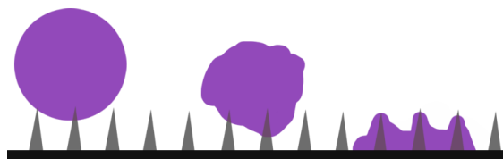
Figure 6. Illustration of the health of Staphylococcus aureus on a nanopillar pattern. Left to right: a healthy, deformed and dead bacterial cell.
