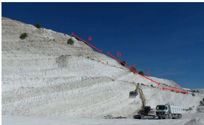
Figure 10.3: Active mine face section of the diatomite deposit where some of the ore samples were obtained: (a) limestone layer with small intercalations of diatomite, (b) diatomite layer with small intercalations of limestones, (c) limestone layer, (d) intercalation of diatomite, limestones, marls and clay horizons, (e) diatomite layer with small intercalations of limestones.
