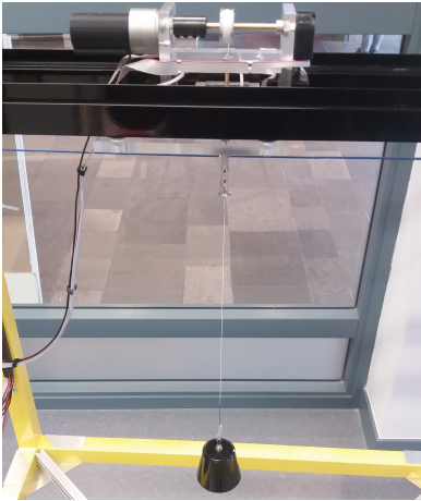
(a) This is a photo of a real experimental set-up showing the load and the mechanism to vary the cable length.
