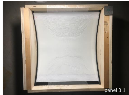
Figure 9.14: Symmetrically combined numerical results at 400 N and experimental crack patterns at failure for panels with an interlayer of SAF (left) and SG (right)
