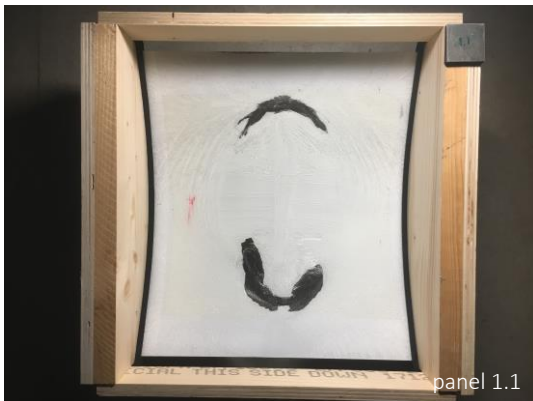
Figure 9.14: Symmetrically combined numerical results at 400 N and experimental crack patterns at failure for panels with an interlayer of SAF (left) and SG (right)
