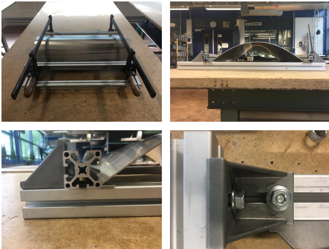
Figure 9.2: Adjustable aluminium mould
