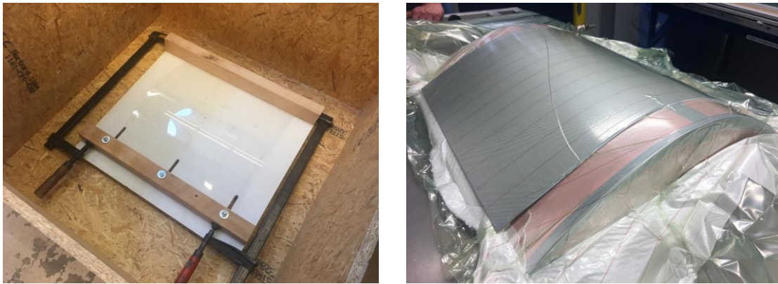
Figure D.1: Adjustable timber mould and nonadjustable aluminium mould
