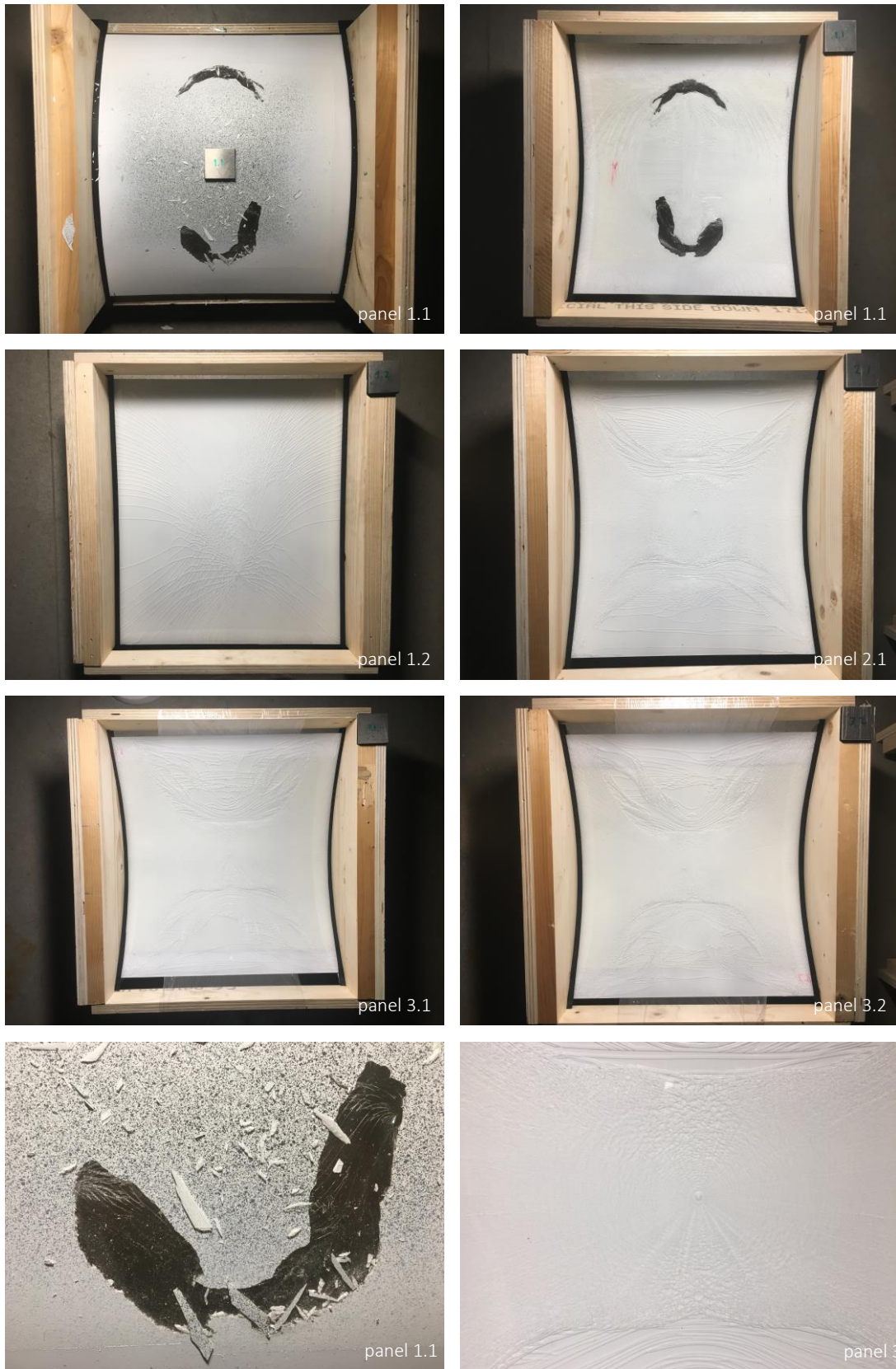
Figure E.27: Crack patterns at failure
