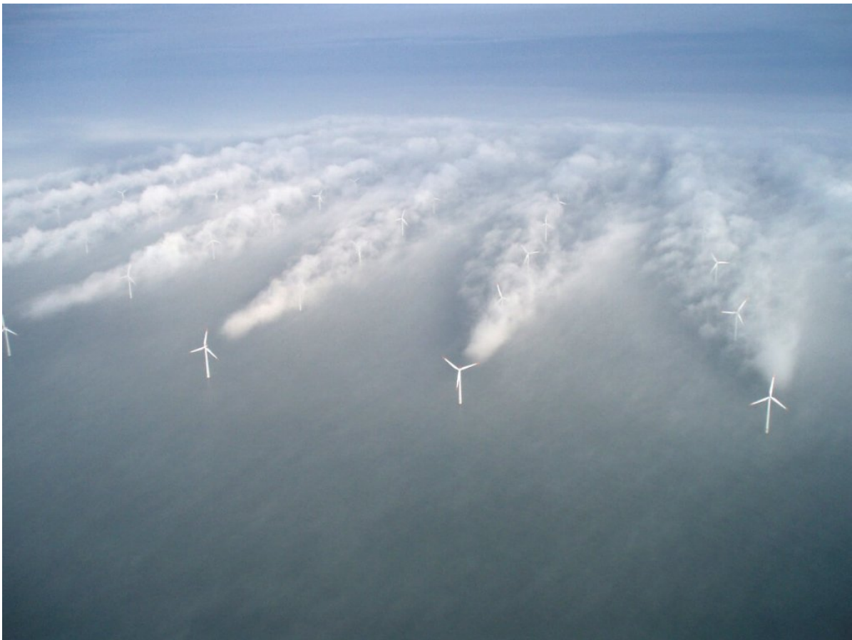
Figure 1.7: Wind farm wake at Horns Rev offshore wind farm in Denmark (Shah, 2016).
