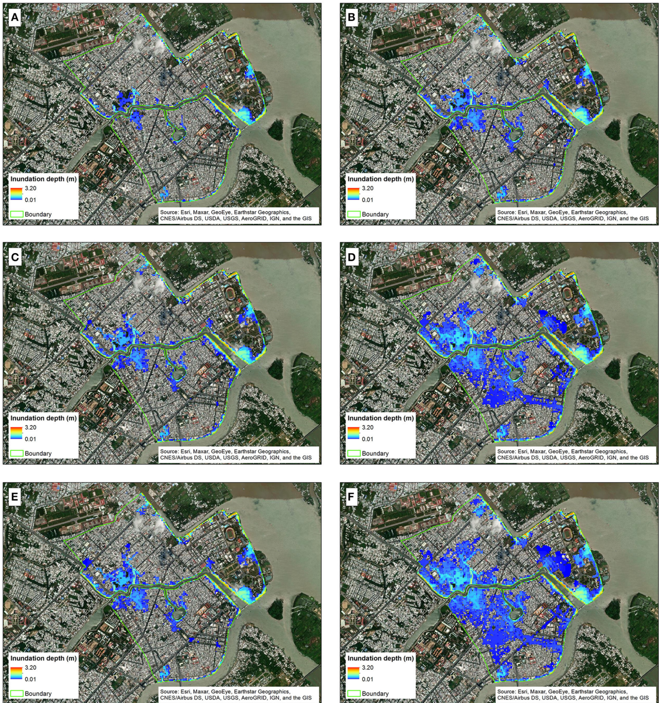
FIGURE 11 | Flood hazard maps corresponding to 5 year and 100 return period of water level for the present (model scenario #1) (A,B), 2050 under RCP 4.5 (model scenarios #3) (C,D), and RCP 8.5 (model scenarios #5) (E,F), respectively.
