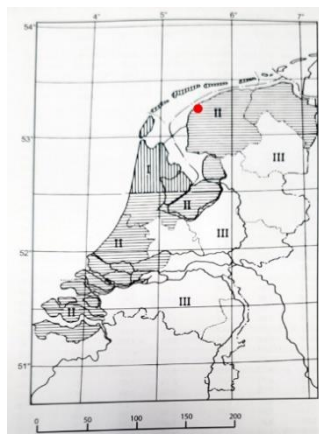
Figure 23: Wind-area map for the Netherlands with Harlingen highlighted by the red dot
