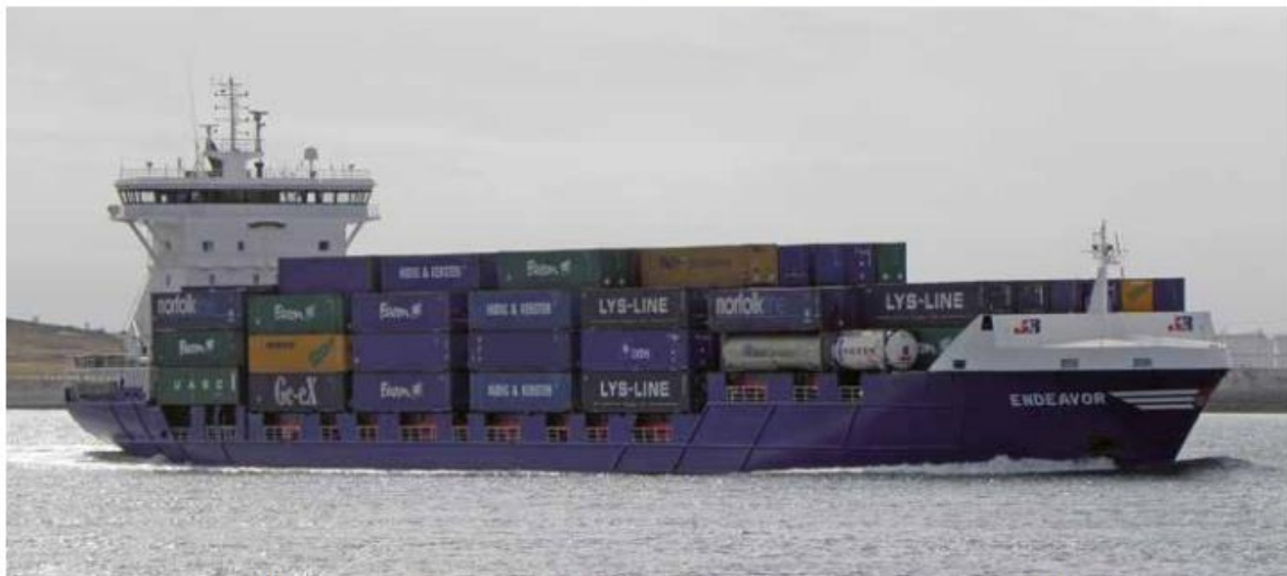
Container vessels with excellent stowage flexibility and a high service speed. Endeavor, Endurance and Ensemble with iceclass E3. Type VH 750. Builder: Volharding Shipyard. Owner: JR Shipping BV.
