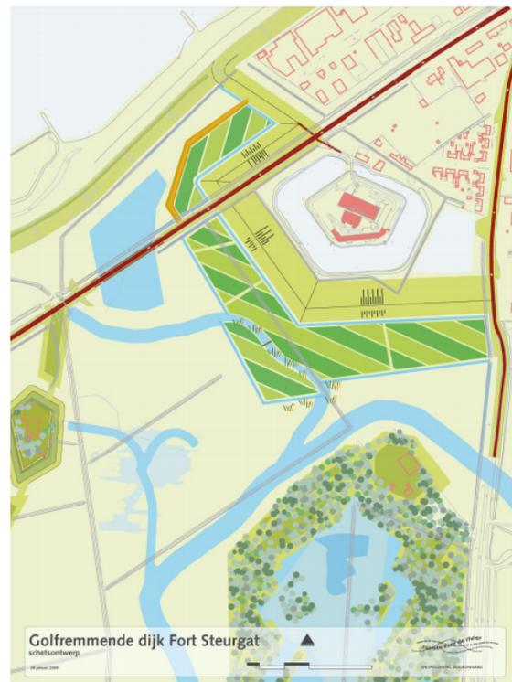
Figure 8.2: Top view of the dike which will reduce the waves at Fort Steurgat (Deltares, 2014)
